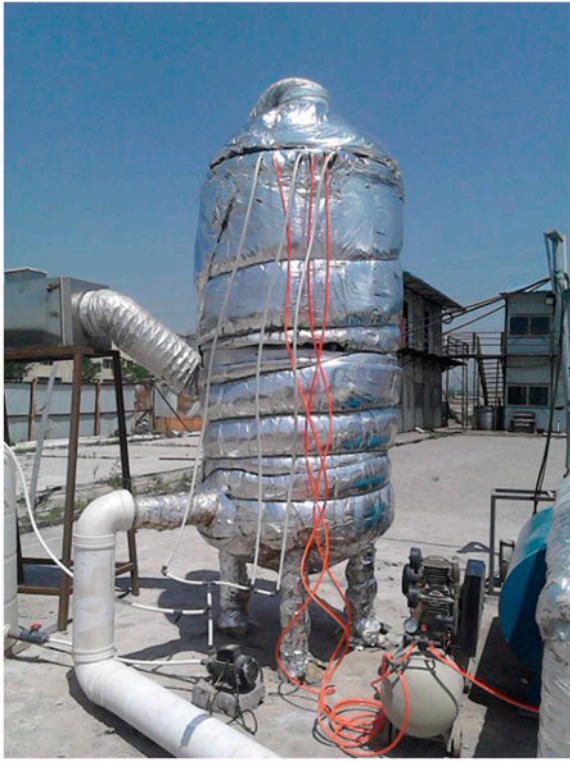
Fig. 2. Appearance of the brine spray tower.
