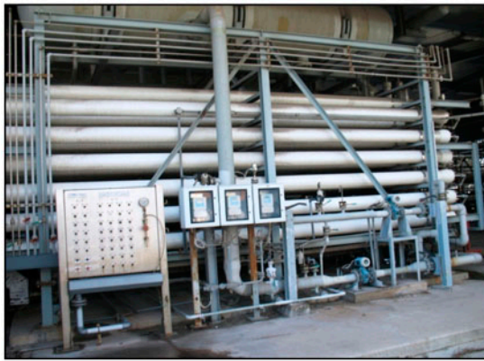
Fig. 3. Typical membrane rack and the two-passes two-steps configuration of the RO section.
