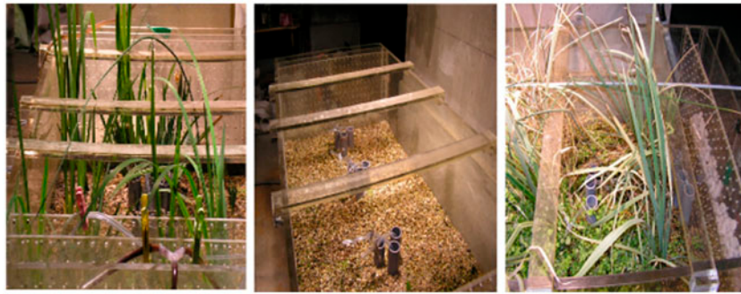
Fig. 1. Planted, aerated at inlet(Case I), non-planted, non-aerated (Case II) and planted, non-aerated (Case III) CW.
