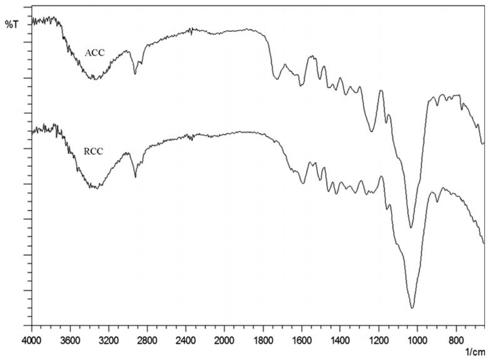
Fig. 2. FTIR spectra of raw and alkali-treated coir.
