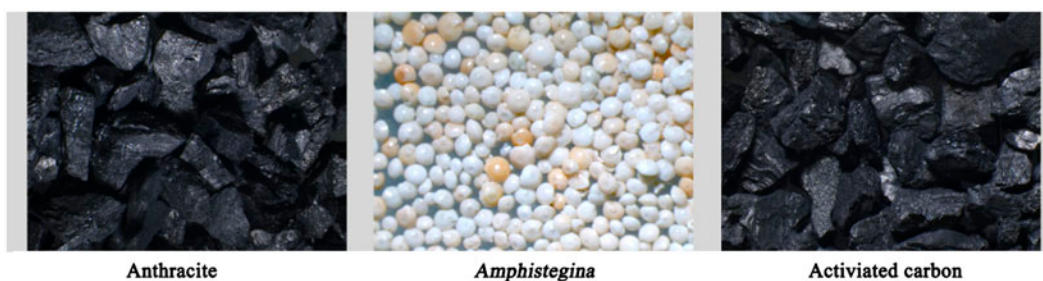
Fig. 2. Pictures of the pretreatment media used in the assembled semi-pilot seawater desalination unit.
