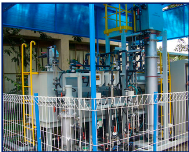
Fig. 1. Pilot-scale membrane filtration unit used in this study.
