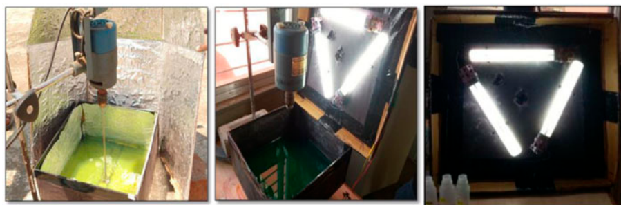
Fig. 2. Experimental set-up for photocatalysis experiments based on UV and solar irradiation.
