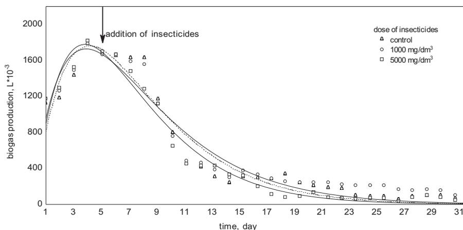
Fig. 2. Gas production during the digestion processes of sludge containing malathion [4,8].
