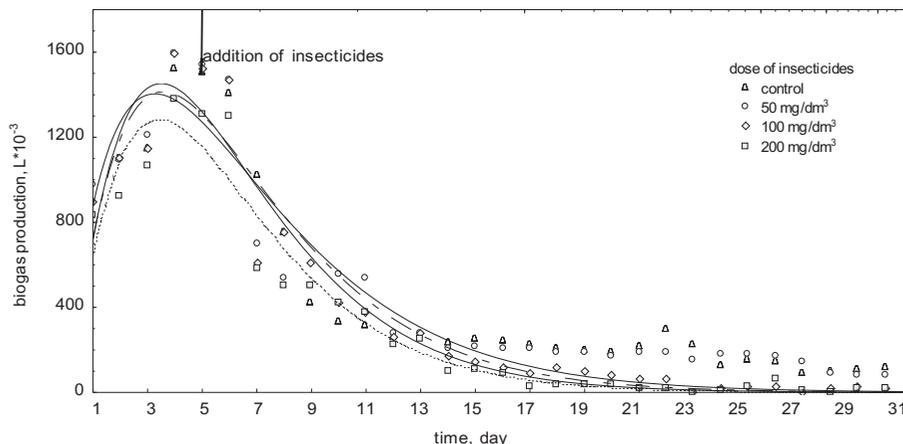
Fig. 1. Gas production during the digestion processes of sludge containing metoxychlor [4,8].
