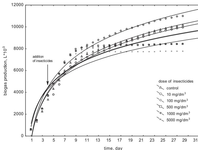
Fig. 3. Production of gas during the digestion process of sludge containing chlorfenvinphos [4,8].
