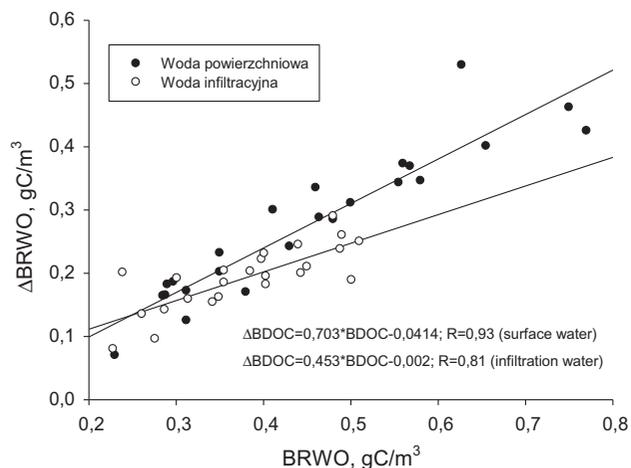
Fig. 3. Influence of the initial content of BDOC content on its reduction in the process of adsorption.
