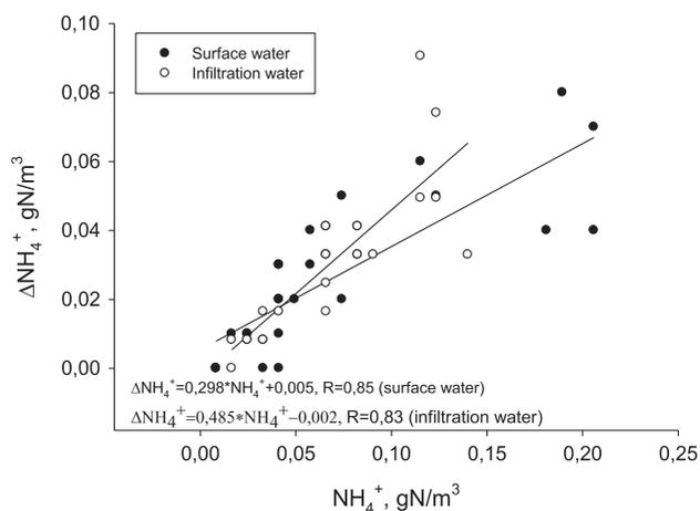
Fig. 6. The influence of the content of ammonium ions in water undergoing biofiltration on its reduction.
