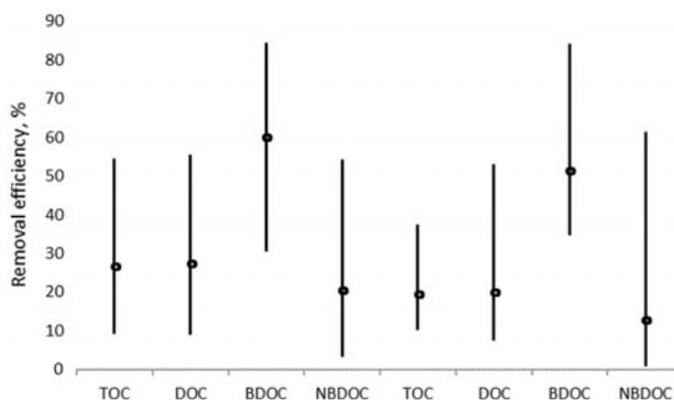
Fig. 5. Range and average efficiency of removal of organic substances fractions.
