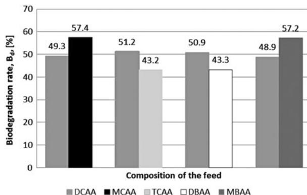
Fig. 4. The impact of the feed composition on DCAA removal rate (the first series of the study).
