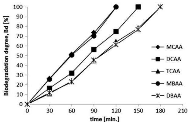
Fig. 1. Dependence of the biodegradation degree of HAAs on duration of process in bioreactor with native enzymes.
