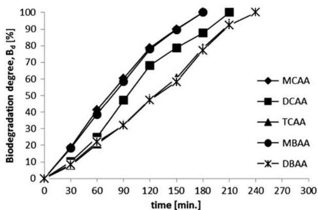
Fig. 2. Dependence of the biodegradation degree of HAAs on duration of process in bioreactor with immobilized enzymes.
