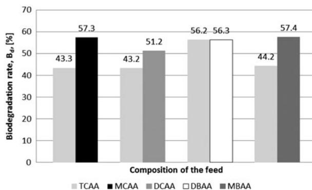
Fig. 5. The impact of the feed composition on TCAA removal rate (the first series of the study).
