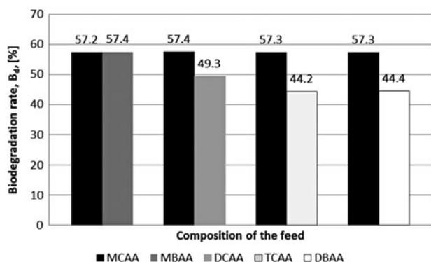
Fig. 3. The impact of the feed composition on DBAA removal rate (the first series of the study).
