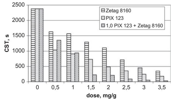
Fig. 7. The effect of chemical reagents dose on CST for ON sludge sonicated for 180 s with  $A = 30.5 \mu\text{m}$ .
