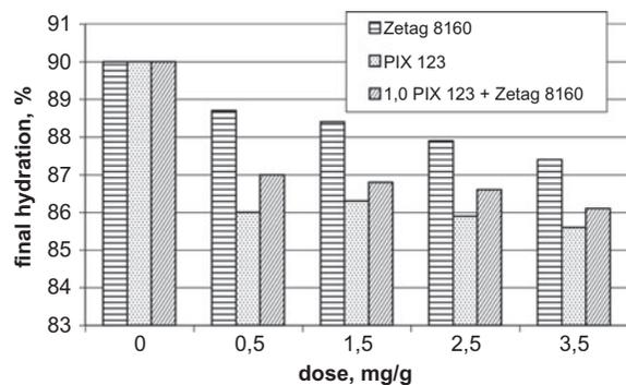
Fig. 11. The effect of chemical reagents dose on the changes of final hydration of ON sludge sonicated within 180 s and with  $A = 15.25 \mu\text{m}$  in the process of pressure filtration.
