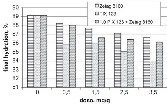
Fig. 10. The effect of chemical reagents dose on the changes of final hydration of ON sludge sonicated within 120 s and with  $A = 15.25 \mu\text{m}$  in the process of pressure filtration.
