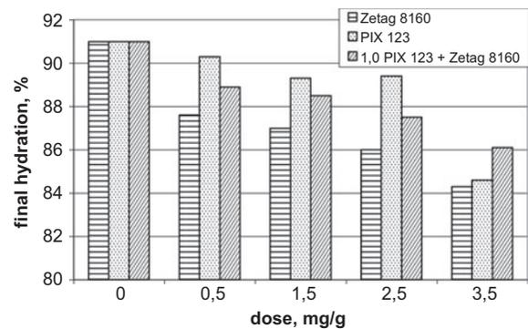
Fig. 8. The effect of chemical reagents dose on the changes of OP sludge final hydration in the process of pressure filtration.
