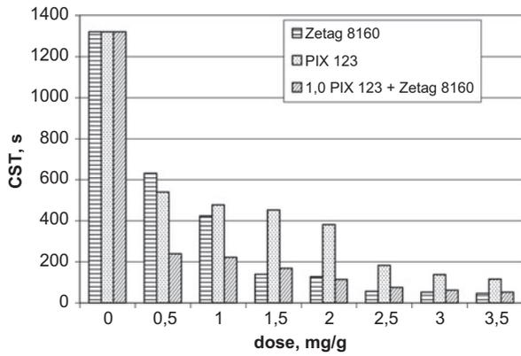
Fig. 3. The effect of chemical reagents dose on CST for ON sludge sonicated for 120 s with  $A = 15.25 \mu\text{m}$ .
