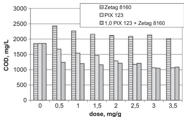
Fig. 18. The effect of chemical reagents dose on the COD of OP sludge supernatant.
