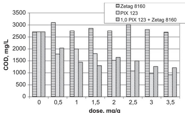
Fig. 19. The effect of chemical reagents dose on the COD of sludge supernatant. ON sludge sonicated for 120 s;  $A = 15.25 \mu\text{m}$ .
