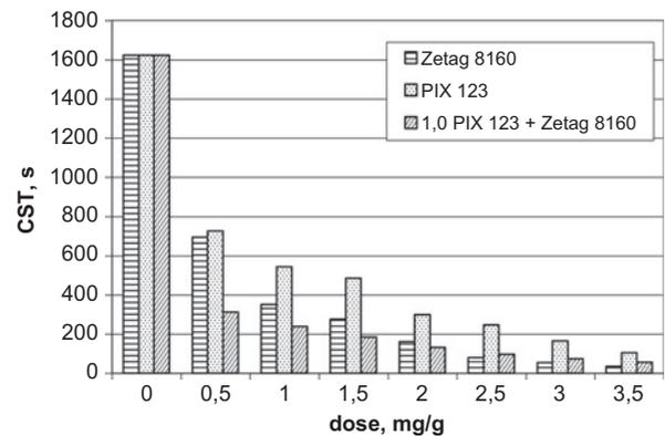
Fig. 2. The effect of chemical reagents dose on CST for ON sludge sonicated for 60 s with  $A = 15.25 \mu\text{m}$ .
