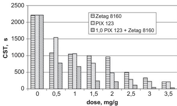
Fig. 5. The effect of chemical reagents dose on CST for ON sludge sonicated for 60 s with  $A = 30.5 \mu\text{m}$ .
