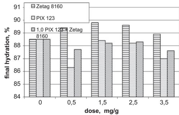
Fig. 12. The effect of chemical reagents dose on the changes of final hydration of ON sludge sonicated within 60 s and with  $A = 30.5 \mu\text{m}$  in the process of pressure filtration.
