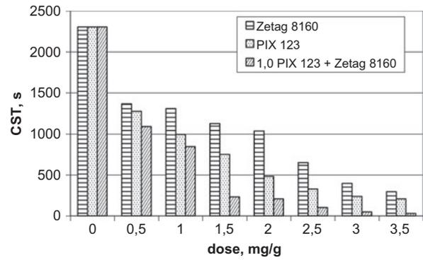
Fig. 6. The effect of chemical reagents dose on CST for ON sludge sonicated for 120 s with  $A = 30.5 \mu\text{m}$ .
