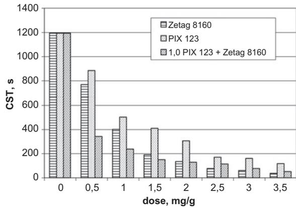
Fig. 4. The effect of chemical reagents dose on CST for ON sludge sonicated for 180 s with  $A = 15.25 \mu\text{m}$ .
