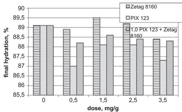
Fig. 13. The effect of chemical reagents dose on the changes of final hydration of ON sludge sonicated within 120 s and with  $A = 30.5 \mu\text{m}$  in the process of pressure filtration.
