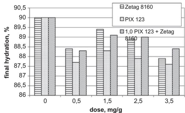
Fig. 14. The effect of chemical reagents dose on the changes of final hydration of ON sludge sonicated within 180 s and with  $A = 30.5 \mu\text{m}$  in the process of pressure filtration.
