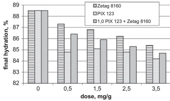
Fig. 9. The effect of chemical reagents dose on the changes of final hydration of ON sludge sonicated within 60 s and with  $A = 15.25 \mu\text{m}$ .
