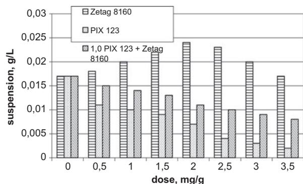
Fig. 17. The effect of chemical reagents dose on the quality of sludge supernatant (ON sludge sonicated for 120 s;  $A = 15.25 \mu\text{m}$ ).
