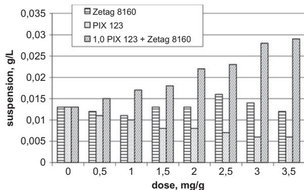
Fig. 16. The effect of chemical reagents dose on the quality of OP sludge supernatant.
