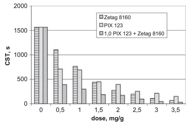
Fig. 1. The effect of chemical reagents dose on CST for OP sludge.
