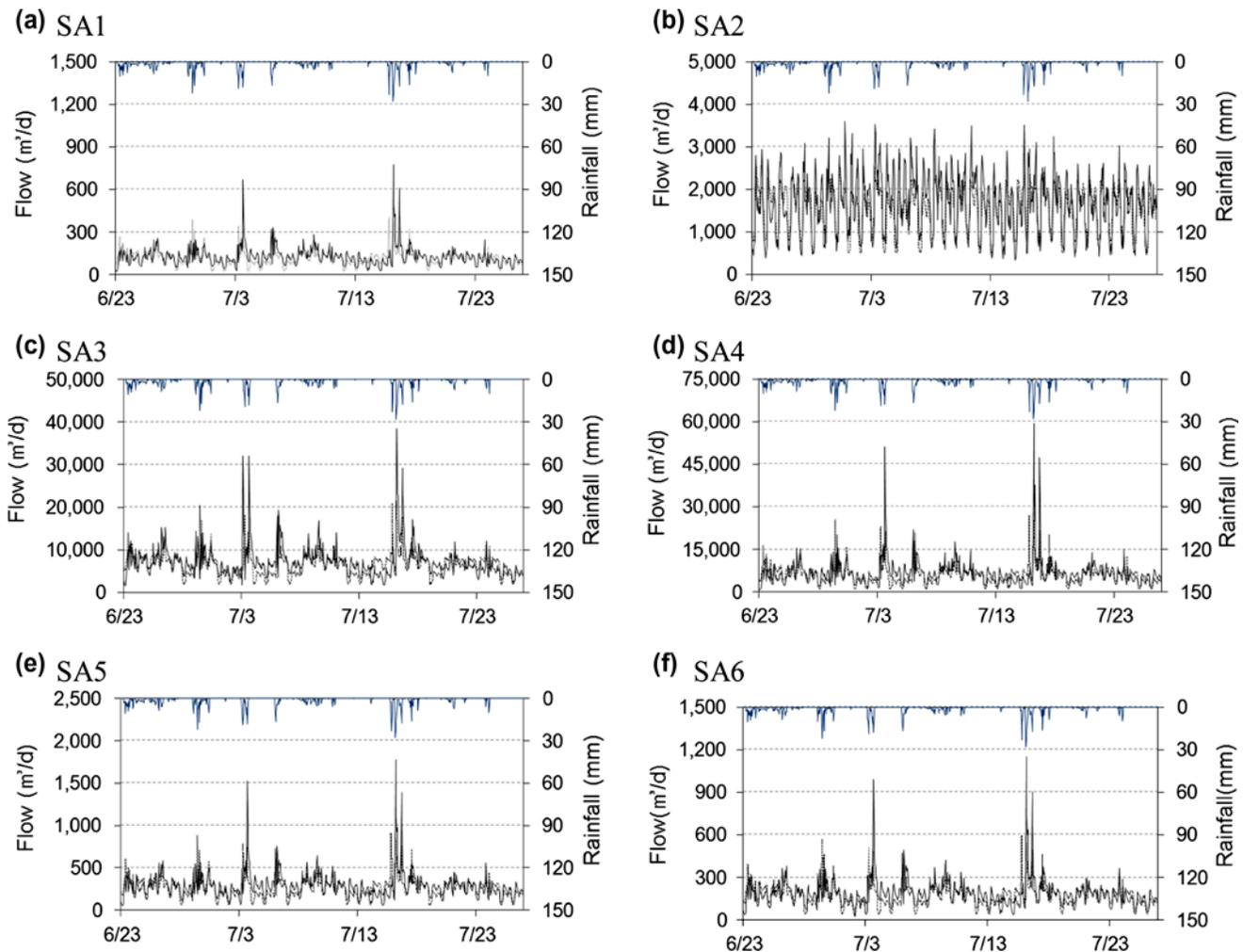
Fig. 4a. Results of model calibration (23 June–23 July 2011, 816 h) (simple line: measured flow, dotted line: modeled flow).
