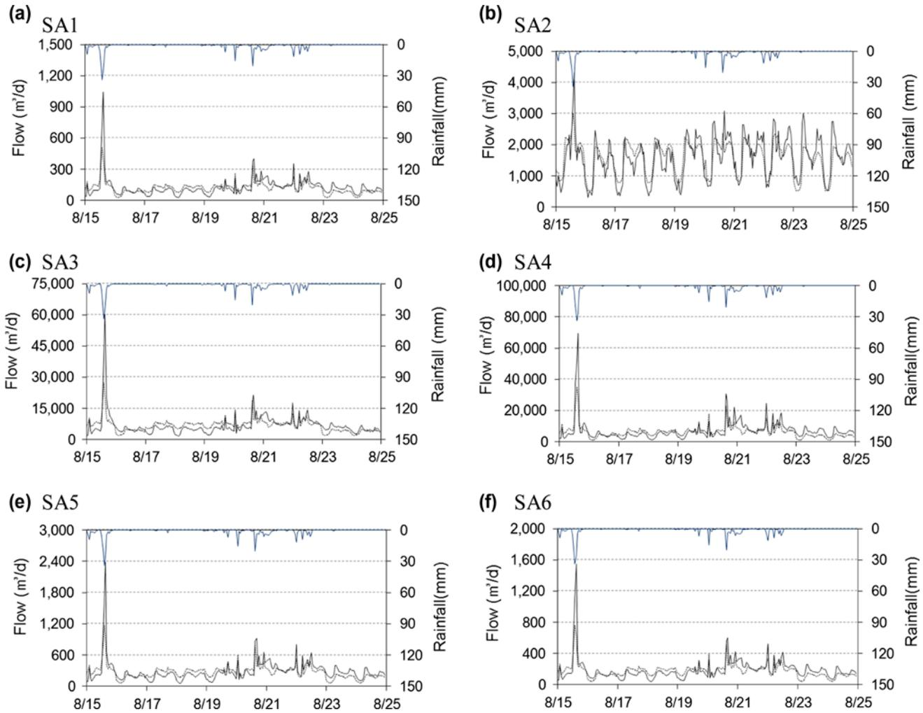
Fig. 4b. Results of model verification (15–24 August 2012, 240 h) (simple line: measured flow, dotted line: modeled flow).
