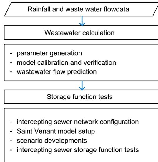
Fig. 3. Framework for testing of storage function of intercepting sewers.
