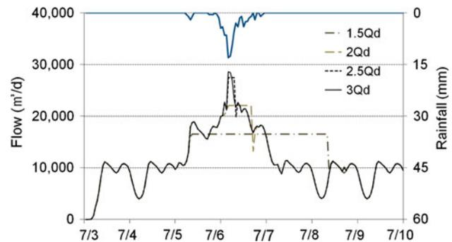
Fig. 5. Hydrographs of inflow to the WWTP under different inflow conditions.
