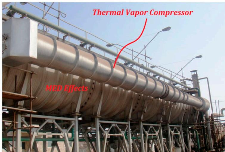
Fig. 2. Experimental setup of MED-TVC.
