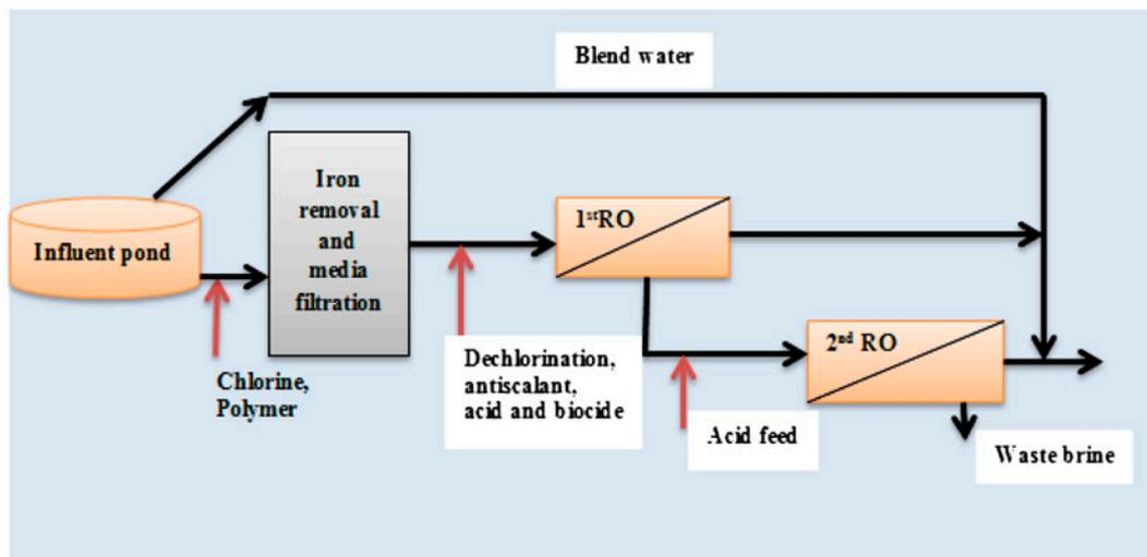
Fig. 6. CSG produced water treatment process in Wild Turkey [64].
