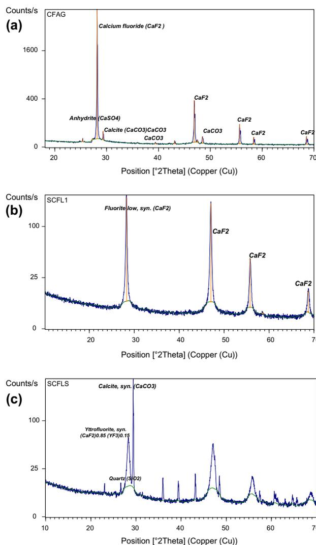
Fig. 4. XRD pattern: (a) Calcium fluoride acid grade ( $\text{CaF}_2 > 97\%$ ); (b) SCFL generated by precipitation–neutralization with lime (SCFL1); (c) SCFL generated by lime stone treatment of AFMW (SCFLS).
