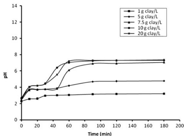
Fig. 10. Effect of clay quantity on the changes in pH with time (initial pH  $2.5 \pm 0.1$ , initial fluoride concentration 167 mg/L and temperature  $25 \pm 1^\circ\text{C}$ ).
