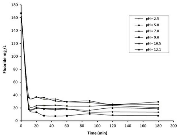
Fig. 11. Effect of initial pH on the changes in fluoride concentration with time (initial pH  $2.5 \pm 0.1$ , initial fluoride concentration  $167 \text{ mg/L}$ , clay mass  $10 \text{ g/L}$ , and temperature  $25 \pm 1^\circ\text{C}$ ).
