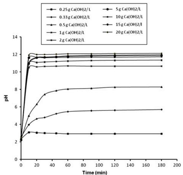
Fig. 2. Effect of lime dose on the changes in pH with time (initial pH  $2.5 \pm 0.1$ , initial fluoride concentration 167 mg/L and temperature  $25 \pm 1^\circ\text{C}$ ).
