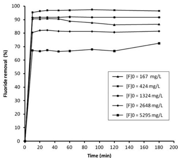
Fig. 3. Effect of fluoride content on the changes in fluoride removal with time (initial  $\text{pH } 2.5 \pm 0.1$ ,  $[\text{Ca}^{2+}]/[\text{F}^-]$  0.8 and temperature  $25 \pm 1^\circ\text{C}$ ).
