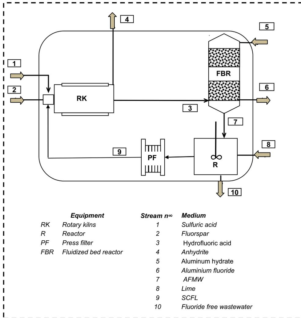
Fig. 5. Scheme of HF and AlF<sub>3</sub> production with integration of SCFL.
