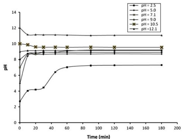
Fig. 12. Changes in pH with time at different pH conditions (initial pH  $2.5 \pm 0.1$ , initial fluoride concentration  $167 \text{ mg/L}$ , clay mass  $10 \text{ g/L}$ , and temperature  $25 \pm 1^\circ\text{C}$ ).
