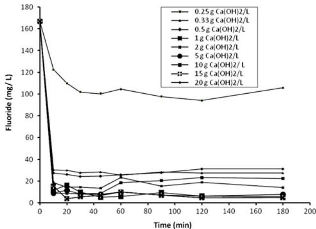
Fig. 1. Effect of lime dose on the changes in fluoride concentration with time (initial pH  $2.5 \pm 0.1$ , initial fluoride concentration 167 mg/L and temperature  $25 \pm 1^\circ\text{C}$ ).
