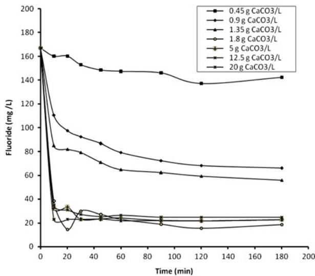
Fig. 6. Effect of limestone dose on the changes in fluoride concentration with time (initial pH  $2.5 \pm 0.1$ , initial fluoride concentration 167 mg/L and temperature  $25 \pm 1^\circ\text{C}$ ).
