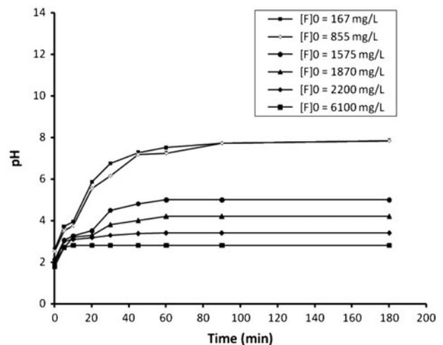
Fig. 8. Effect of fluoride concentration on the evolution with time of pH medium (pH  $2.5 \pm 0.1$ ,  $[\text{Ca}^{2+}]/[\text{F}^-]$  2 and temperature  $25 \pm 1^\circ\text{C}$ ).
