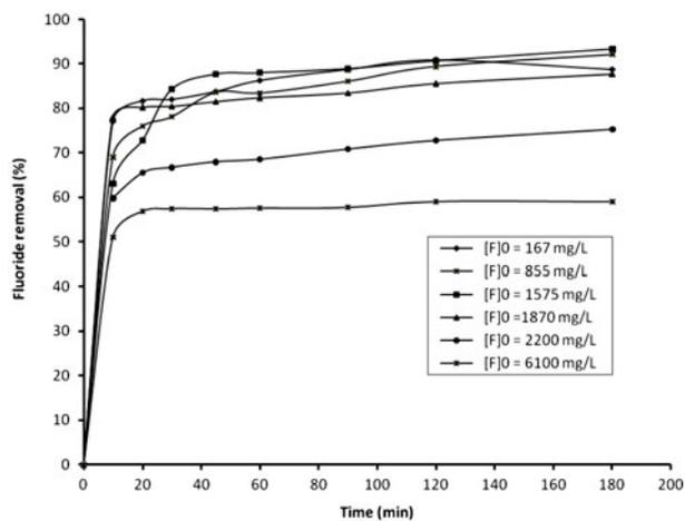
Fig. 7. Effect of fluoride concentration on the changes in fluoride removal with time (initial pH  $2.5 \pm 0.1$ ,  $[\text{Ca}^{2+}]/[\text{F}^-]$  2, and temperature  $25 \pm 1^\circ\text{C}$ ).
