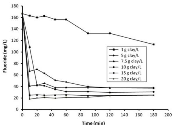
Fig. 9. Effect of clay quantity on the changes in fluoride concentration with time (initial pH  $2.5 \pm 0.1$ , initial fluoride concentration 167 mg/L, and temperature  $25 \pm 1^\circ\text{C}$ ).
