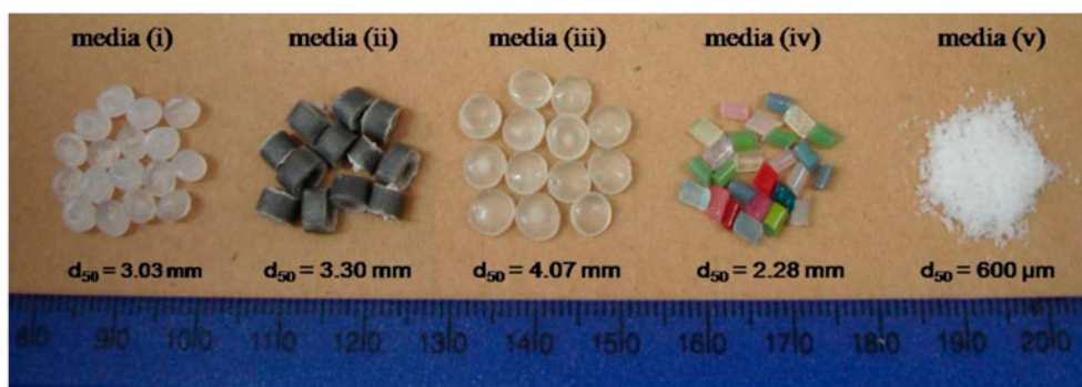
Fig. 2. Different sizes and shapes of plastic media that were tested in this study. From left to right: smooth cubic (media (i)), large cubic (media (ii)), disc (media (iii)), small lice-cut cubic (media (iv)), and LLDPE powder (media (v)).
