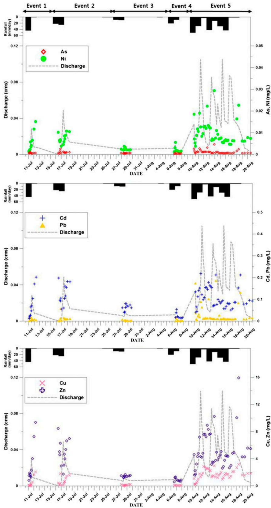
Fig. 4. Variation of dissolved metal concentrations during wet weather at GP-1.
