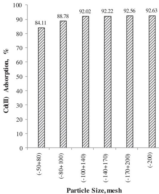
Fig. 4. The effect of particle size on the Cd(II) adsorption by grape stalk [Cd(II) concentration: 10 mg/L; adsorbent dosage: 10 g/L; pH 6; contact time: 60 min; and temperature: 25°C].
