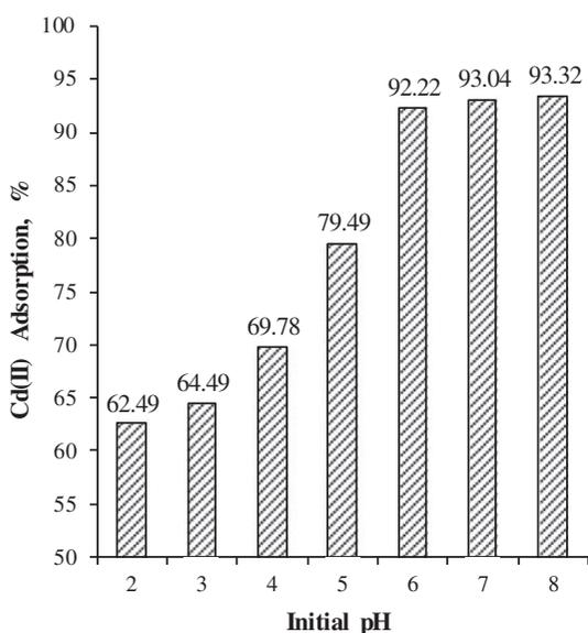
Fig. 3. The effect of pH on the Cd(II) adsorption by grape stalk [Cd(II) concentration: 10 mg/L; adsorbent dosage: 10 g/L; contact time: 60 min; particle size:  $-100 + 140$  mesh; and temperature: 25 °C].
