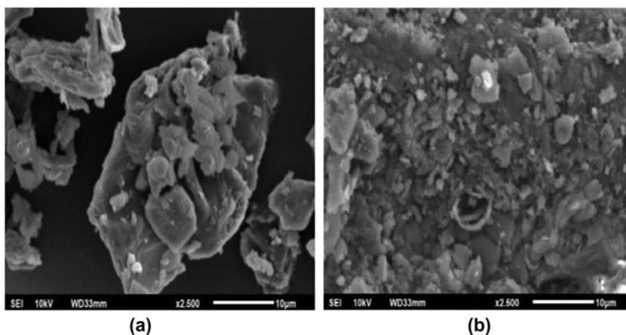
Fig. 2. SEM micrographs of grape stalk (a) and grape stalk loaded with Cd(II) (b).
