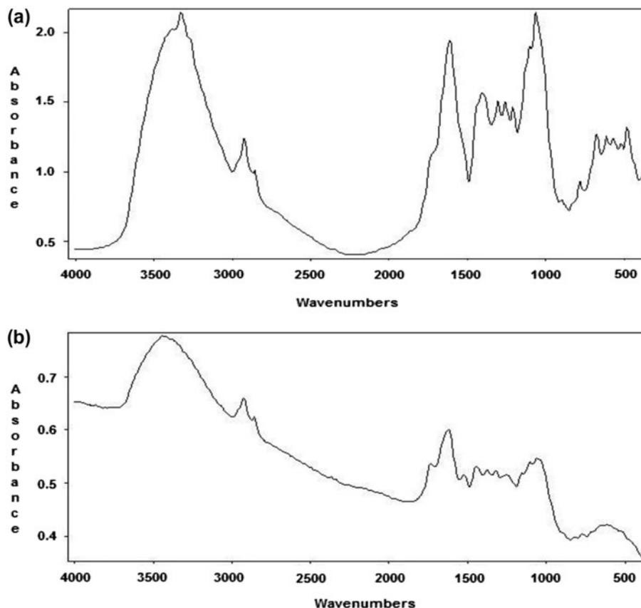
Fig. 1. FTIR spectra of grape stalk (a) and grape stalk loaded with Cd(II) (b).
