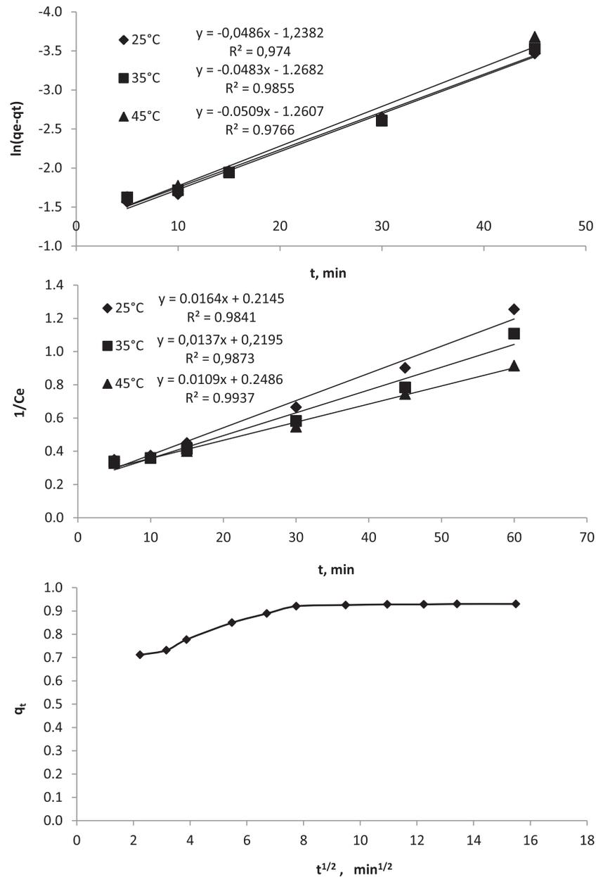
Fig. 7. Lagergren's pseudo-first-order and second-order kinetic model for the adsorption of Cd(II) onto grape stalk [Cd(II) concentration: 10 mg/L; initial pH 6; adsorbent dosage: 10 g/L].
