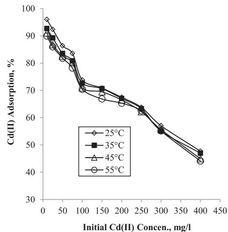
Fig. 6. The effects of initial Cd(II) concentration and temperature on the Cd(II) adsorption by grape stalk [adsorbent dosage: 10 g/L; contact time: 60 min; and particle size:  $-100 + 140$  mesh].
