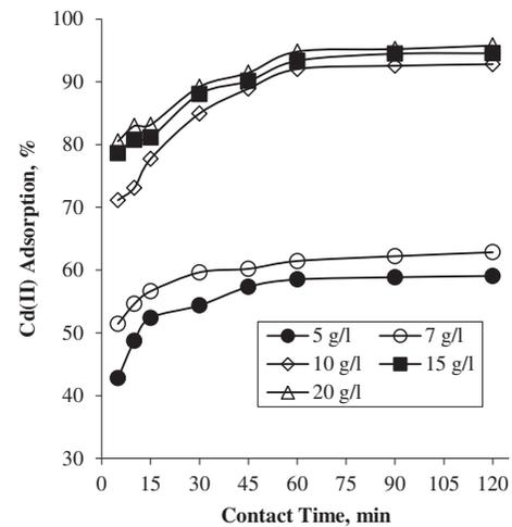
Fig. 5. The effects of adsorbent dosage and contact time on the Cd(II) adsorption by grape stalk [Cd(II) concentration: 10 mg/L; pH 6; particle size:  $-100 + 140$  mesh; and temperature: 25°C].
