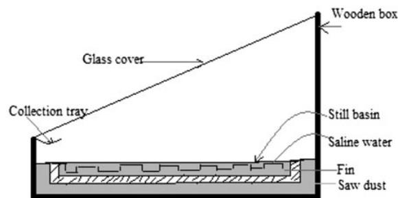
Fig. 3. Cross-sectional view of solar still with fins, taken from Ref. [10].
