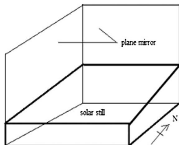
Fig. 5. Twin reflector booster applied to solar still, taken from Ref. [14].
