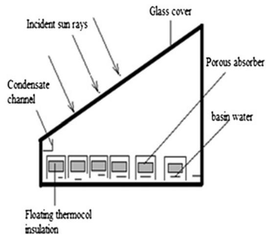
Fig. 4. Construction of the modified still, taken from Ref. [14].
