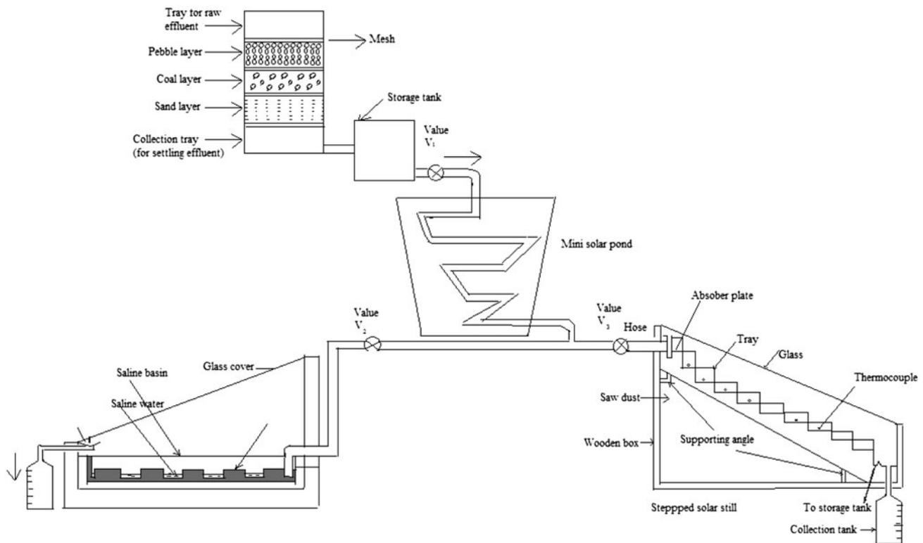
Fig. 1. Schematic diagram of the experimental set-up, taken from Ref. [5].
