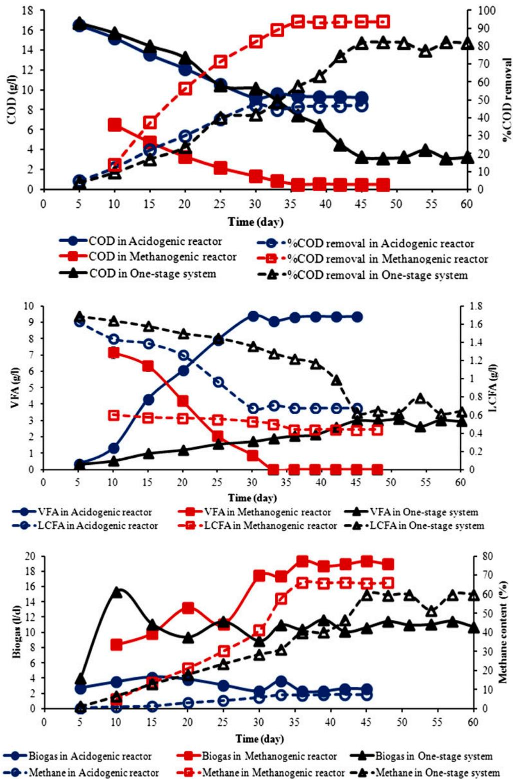
Fig. 4. The profiles of the COD, VFA, LCFA, biogas, and methane content during the anaerobic digestion of the two-stage system (circle symbol for acidogenic reactor and square symbol for methanogenic reactor) and the one-stage system (triangle symbol).
