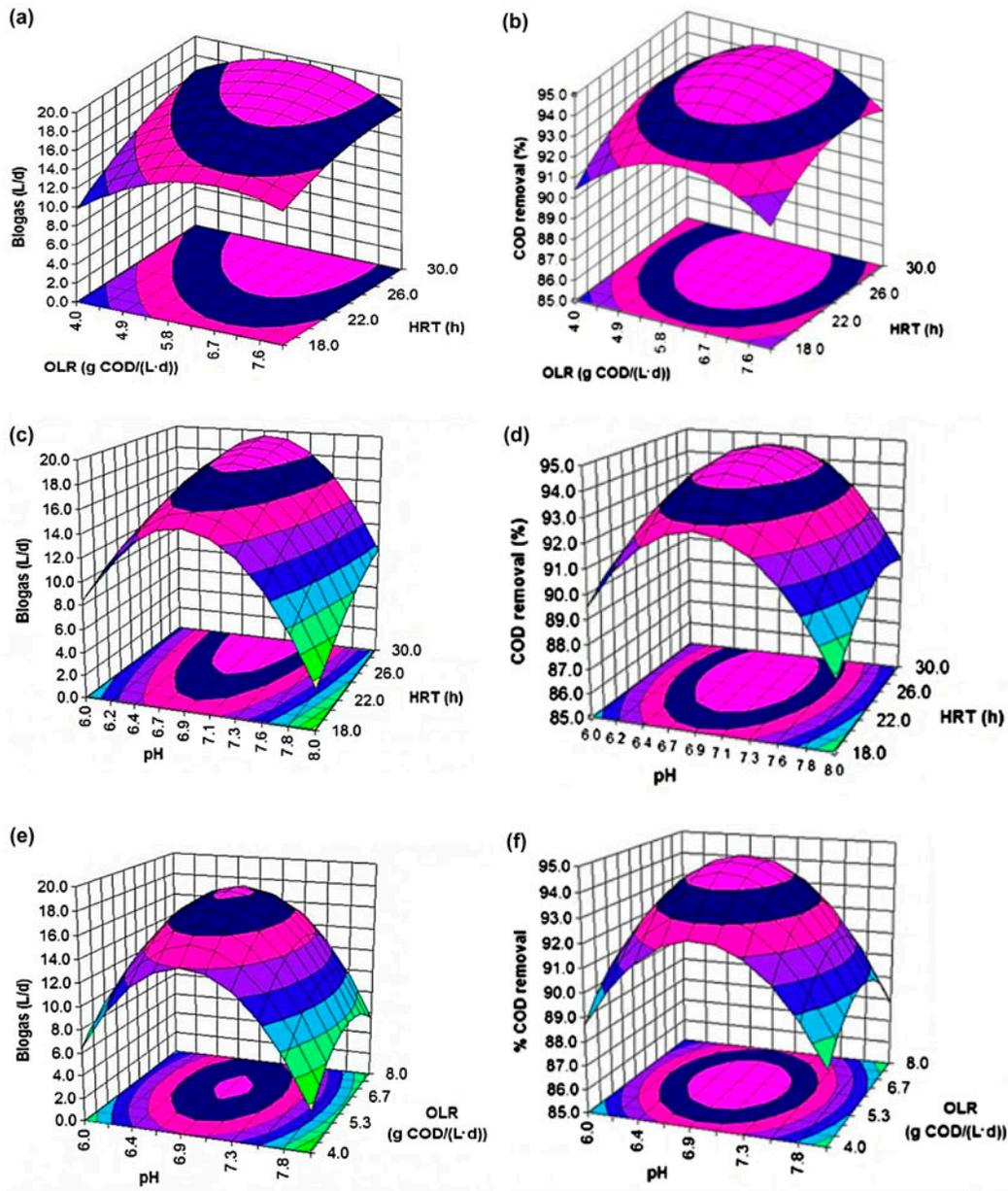
Fig. 3. The 3D response surface for the effect of pH, HRT, and OLR on biogas production ((a), (c), (e)) and COD removal ((b), (d), (f)) in methanogenic reactor.
