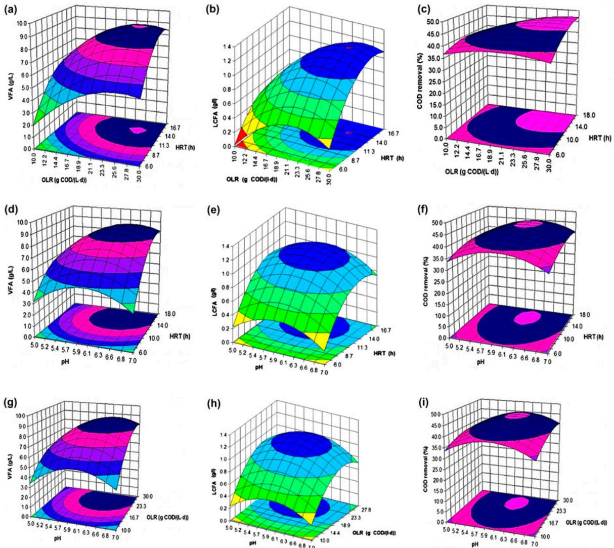
Fig. 2. The 3D response surface for the effect of pH, HRT, and OLR on VFA production ((a), (d), (g)), LCFA consumption ((b), (e), (h)) and COD removal ((c), (f), (i)) in acidogenic reactor.
