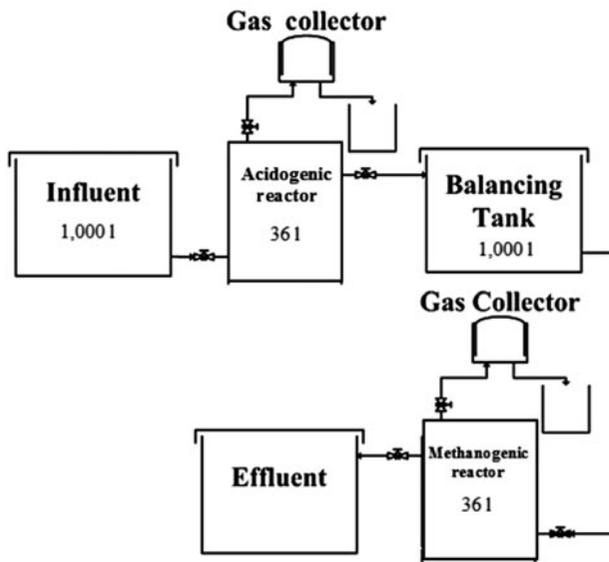
Fig. 1. Schematic diagrams of two-stage anaerobic system.
