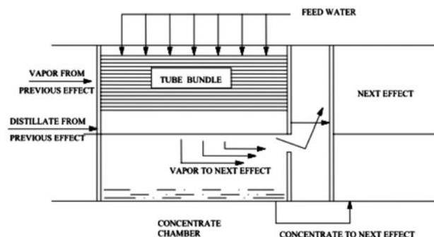
Fig. 1. MEE horizontal tube arrangement [11].
