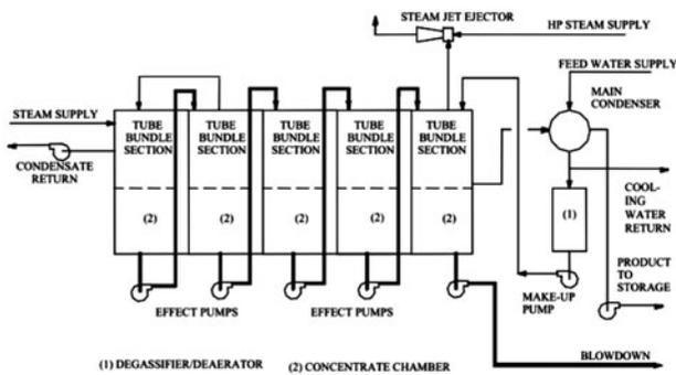
Fig. 2. MEE process schematic—horizontal tube arrangement [11].
