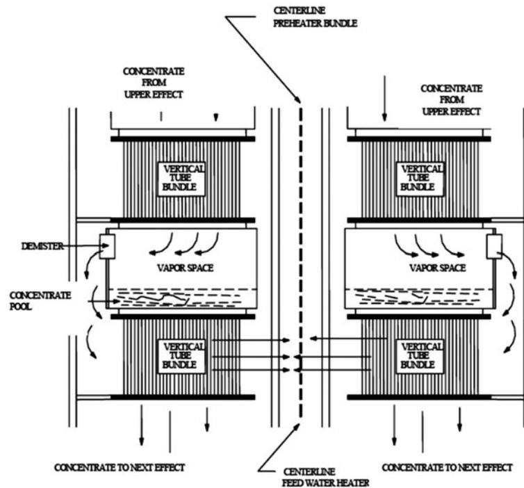
Fig. 4. MEE vertically stacked tube bundles [11].
