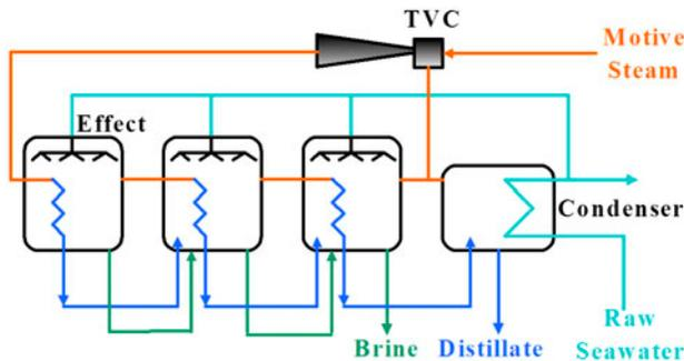
Fig. 5. Schematic diagram of a three-effect ME-TVC plant.
