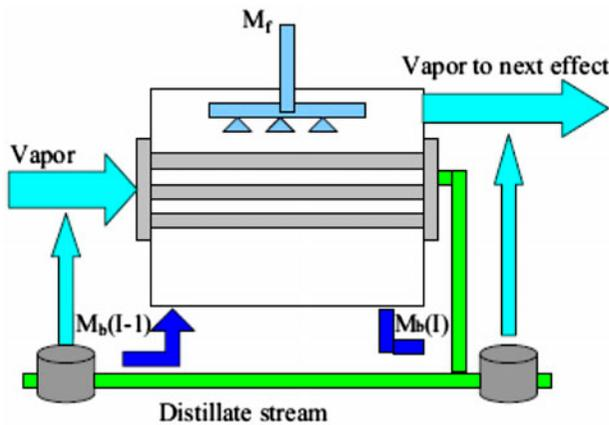
Fig. 6. Evaporator schematic diagram.
