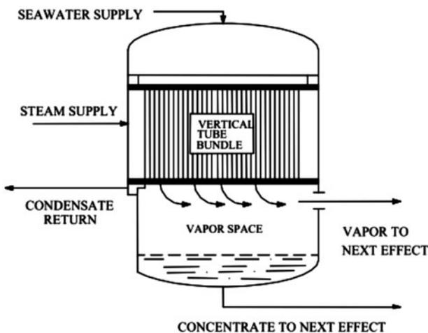
Fig. 3. MEE vertical tube bundle arrangement [11].
