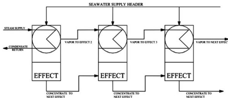
Fig. 7. Three effects of a multiple-effect evaporator [11].
