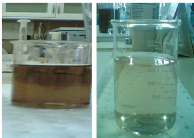
Fig. 3. Appearance of raw and treated wastewaters followed by coagulation experiments.
