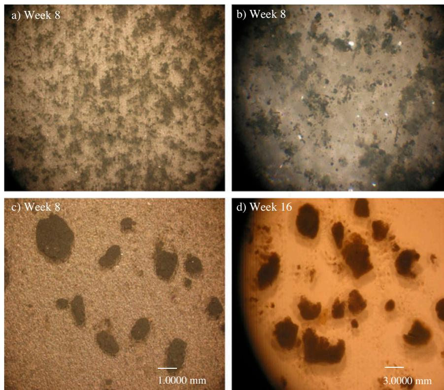
Fig. 2. Images of seed sludge at (a) initial stage (b) after two weeks (c) after eight weeks and (d) after sixteen weeks of granules development under stereo microscopic observation (6.3× magnification).
