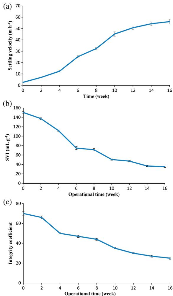
Fig. 3. (a) SV (b) SVI and (c) IC profile of the developed granules.
