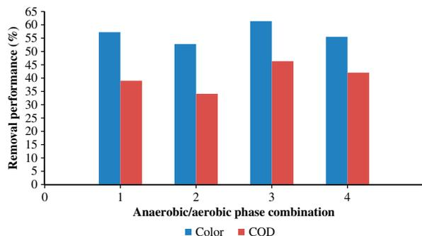
Fig. 7. ADMI and COD removal profile of raw textile wastewater on different combination of anaerobic/aerobic phase: 1: 12 h anaerobic, 12 h aerobic; 2: 15 h anaerobic, 9 h aerobic; 3: 18 h anaerobic, 6 h aerobic; 4: 21 h anaerobic, 3 h aerobic.
