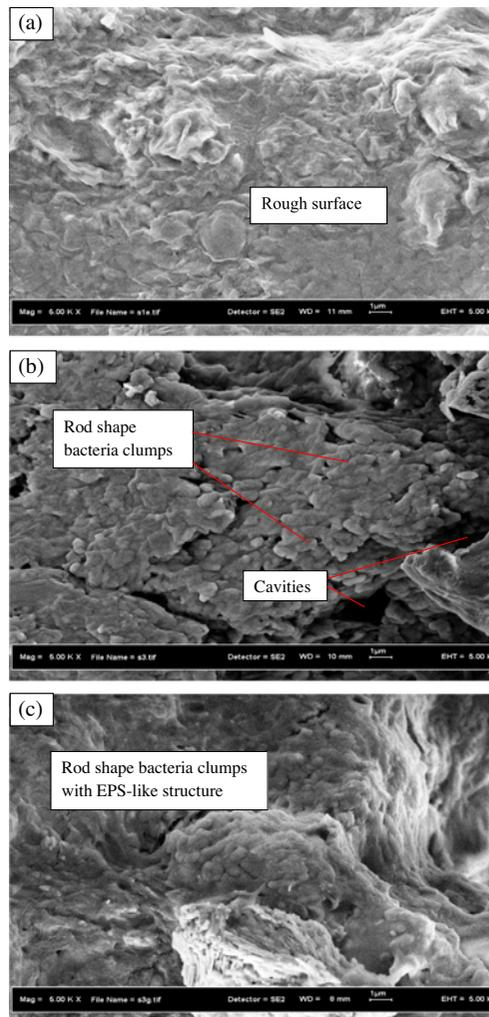
Fig. 4. FESEM observations on (a) surface of initial sludge (b) cross section surface of granules after sixteen weeks and (c) surface of granules after sixteen weeks (5000 $\times$  magnification).
