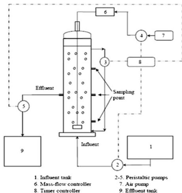
Fig. 1. Schematic diagram of lab-scale SBR system.
