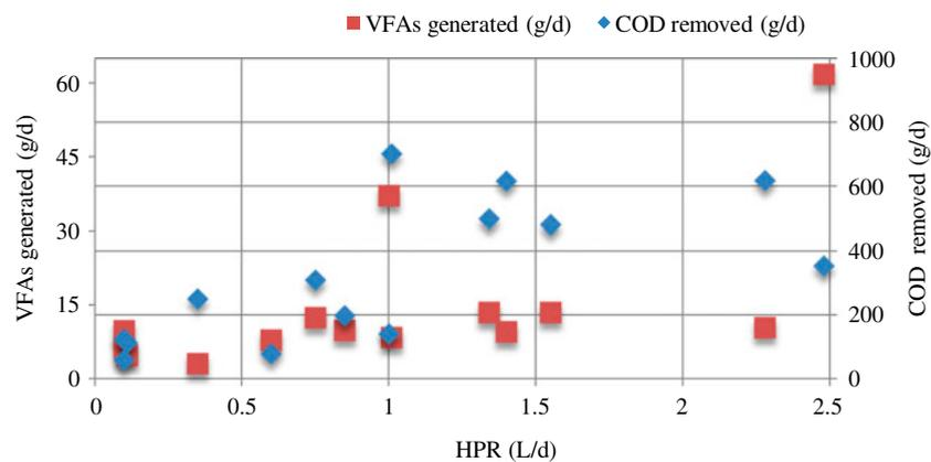
Fig. 4. The relationship between H<sub>2</sub> production rate HPR, COD<sub>removed</sub>, and VFAs<sub>generated</sub>.
