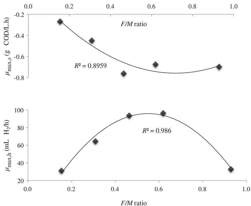
Fig. 7. Effect of  $F/M$  ratios on (a) maximum substrate utilization rate ( $\mu_{\max,s}$ ): and (b) maximum volumetric HPR ( $\mu_{\max,h}$ ).
