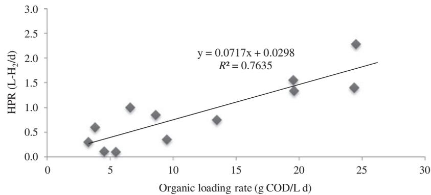
Fig. 3. Effect of OLR on HPR in UASR treating starch processing wastewater industry.
