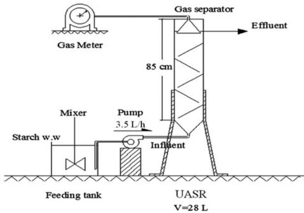
Fig. 1. Schematic diagram of the UASR treating starch wastewater industry.
