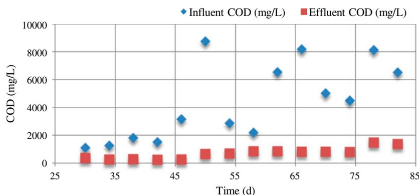
Fig. 2. Time course of COD concentrations in the UASR fed with starch wastewater at a HRT of 8 h.
