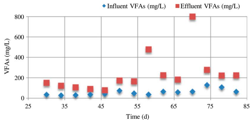
Fig. 5. VFAs generation in UASR treating starch wastewater.
