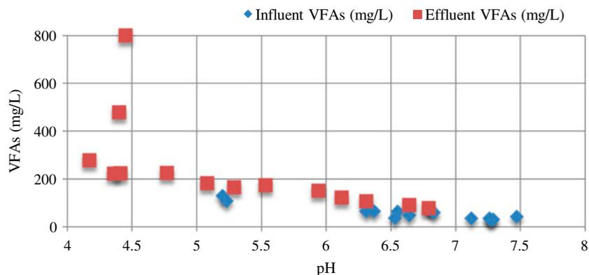
Fig. 6. Correlation between pH and VFAs generation in UASR treating starch wastewater.
