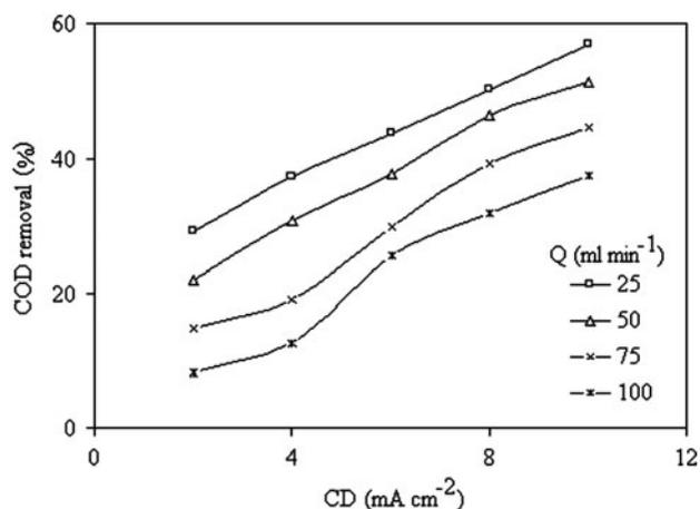
Fig. 2. Effect of effluent flow rate on percentage COD removal.
