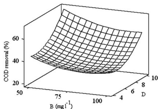
Fig. 6. Response surface plot of initial dye concentration and pH on percentage COD removal. Flow rate:  $25 \text{ ml min}^{-1}$ ; current density:  $6 \text{ mA cm}^{-2}$ .
