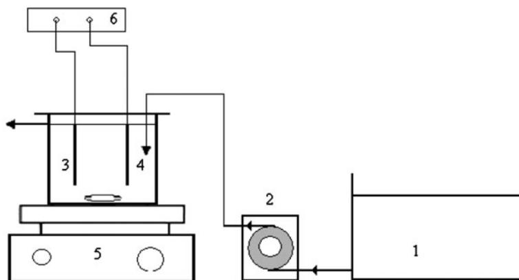
Fig. 1. Schematic representation of CSTER; (1) effluent storage tank; (2) peristaltic pump; (3) anode; (4) cathode; (5) magnetic stirrer; and (6) DC power supply.
