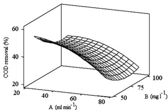
Fig. 4. Response surface plot of flow rate and initial dye concentration on percentage COD removal. Current density:  $6 \text{ mA cm}^{-2}$ ; pH 7.0.
