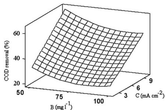
Fig. 5. Response surface plot of initial dye concentration and current density on percentage COD removal. Flow rate:  $25 \text{ ml min}^{-1}$ ; pH 7.0.
