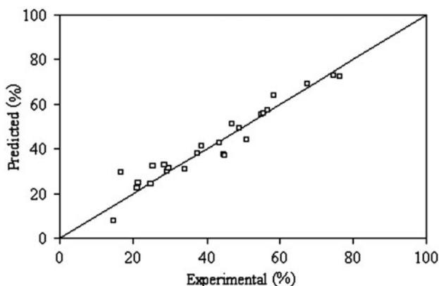
Fig. 3. Comparison of model prediction with experimental observations on percentage COD removal.
