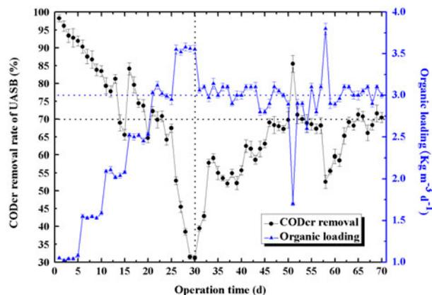
Fig. 3. The removal effect of UASB on CODcr.
