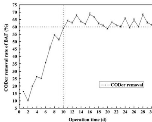
Fig. 5. The removal effect of BAF on COD<sub>Cr</sub>.
