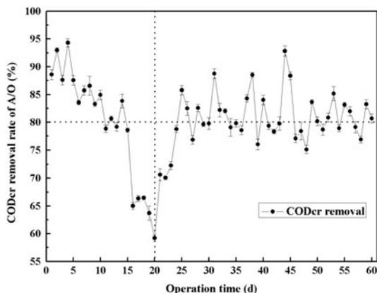
Fig. 4. COD<sub>Cr</sub> removal effect of A/O.
