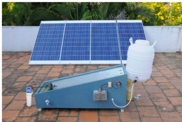
Fig. 7. Vacuum solar still with solar inverter.
