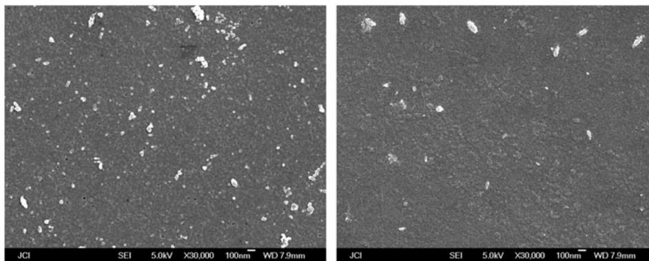
Fig. 8. The SEM images of the UF membrane and NF membrane (left, UF; right, NF).
