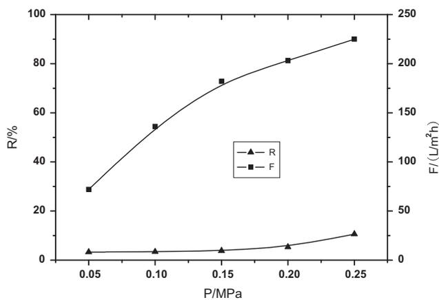
Fig. 4. Effect of operation pressure on the PEI UF membrane performance.
