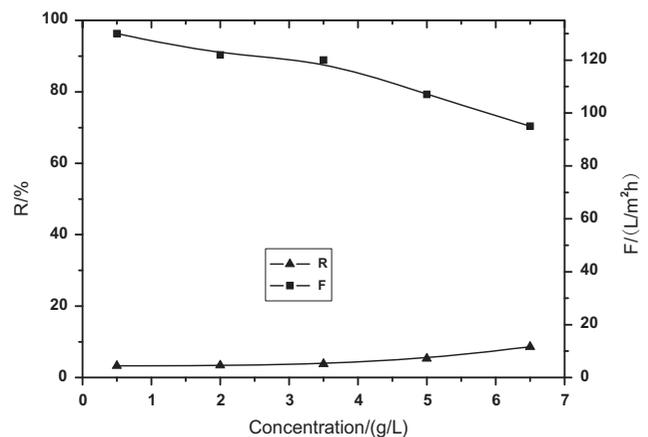
Fig. 5. Effect of feed concentration on the PEI UF membrane performance.
