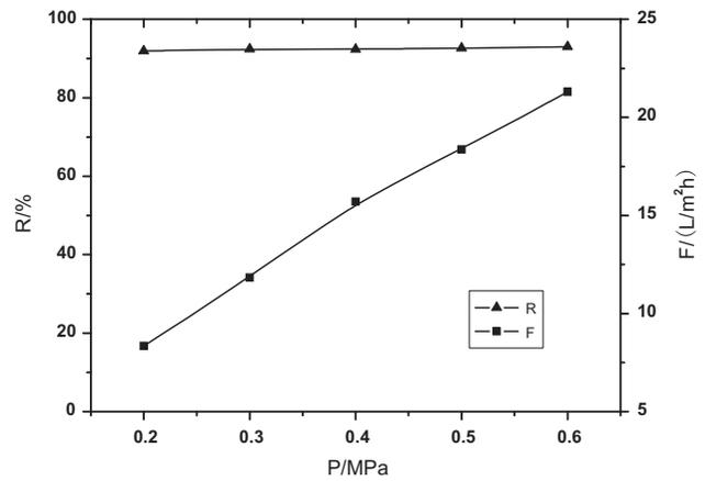
Fig. 6. Effect of operation pressure on the NF membrane performance.
