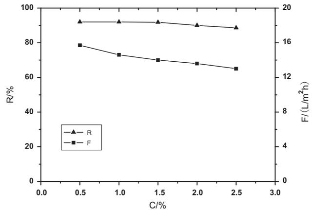
Fig. 7. Effect of feed concentration on the NF membrane performance.
