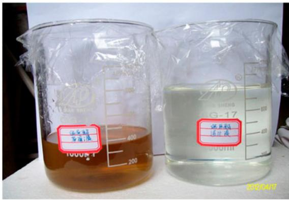
Fig. 3. The decoloration effect of the PEI UF membrane.
