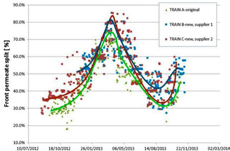
Fig. 5. Front permeate split, original membranes (Train A) vs. new-generation membranes (Trains B and C).
