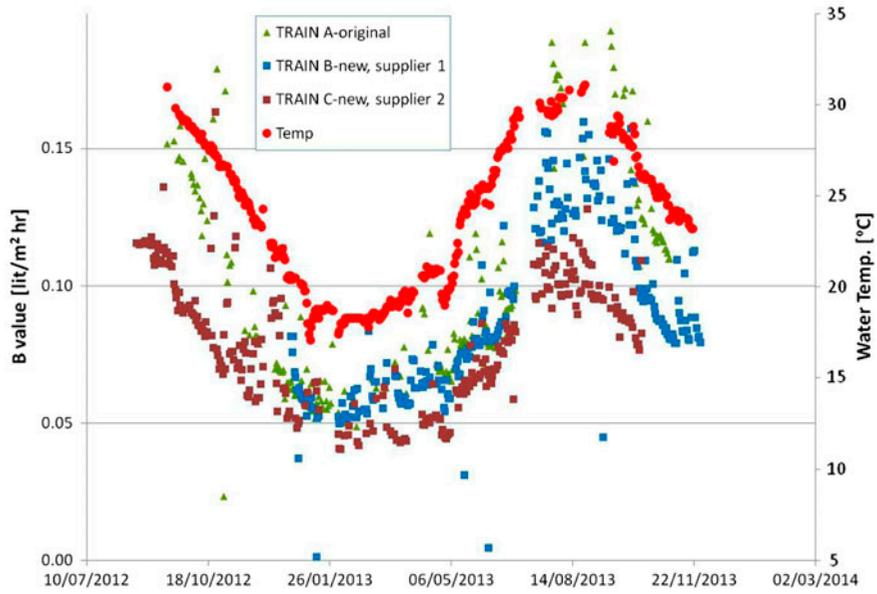
Fig. 6. Salt passage *B* value, original membranes (Train A) vs. new-generation membranes (Trains B and C).
