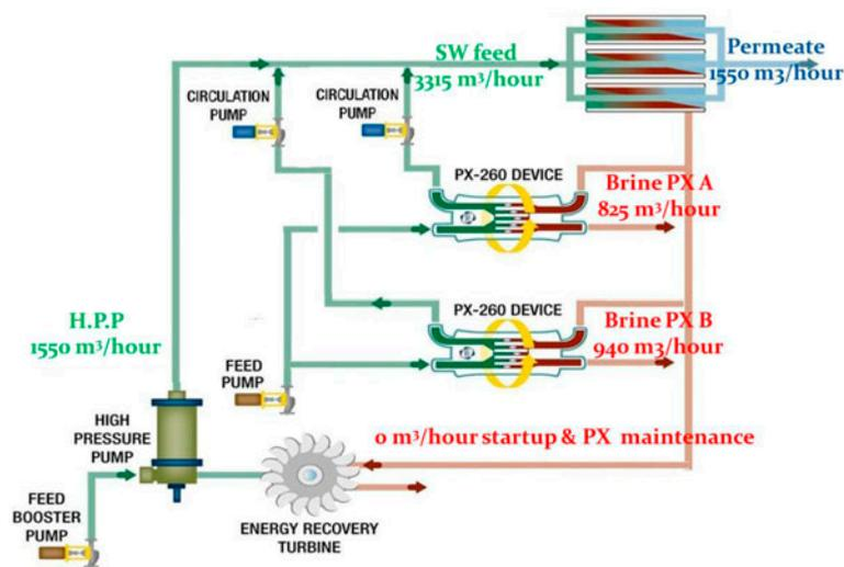
Fig. 2. Palmachim desalination plant—new expanded RO power scheme.
