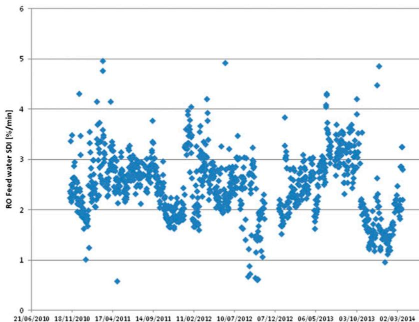
Fig. 1. Palmachim desalination plant—RO feed water SDI.
