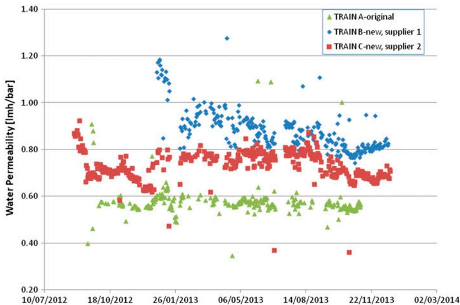
Fig. 3. Membrane permeability, original membranes (Train A) vs. new-generation membranes (Trains B and C).
