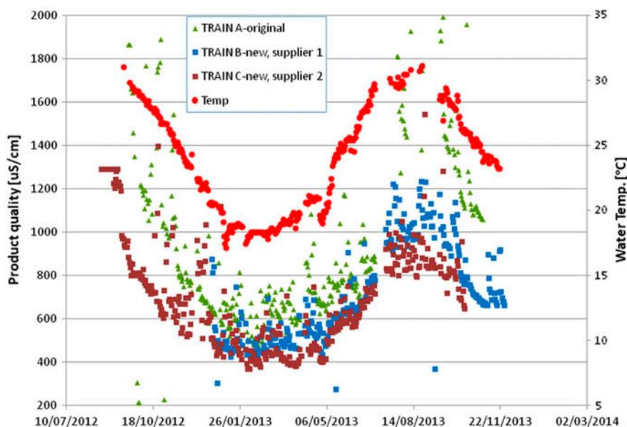
Fig. 4. Permeate quality, original membranes (Train A) vs. new-generation membranes (Trains B and C).
