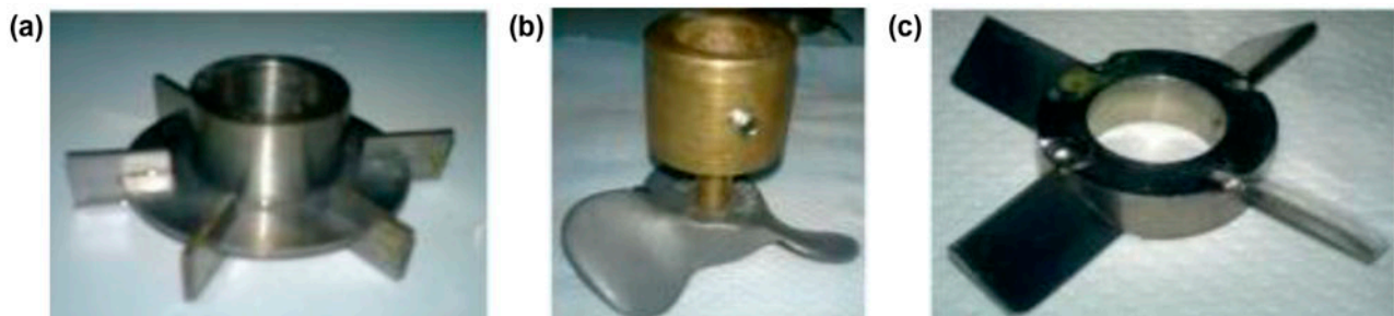
Fig. 3. The three impellers adopted in the semi-batch experiments. (a) Rushton turbine; (b) marine propeller; and (c) pitched-blade impeller.
