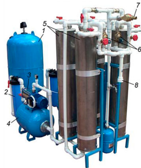
Fig. 3. Nanofiltration unit for surface water treatment: 1—pressure feed water tank; 2—prefilter 50–100 micron; 3—feed water pump; 4—flush water tank; 5—nanofiltration modules; 6—solenoid valves; 7—clean water outlet; 8—concentrate and flush water discharge.
