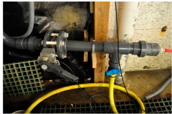
Fig. 5. Photograph of the 316L butterfly valve in the set-up.
