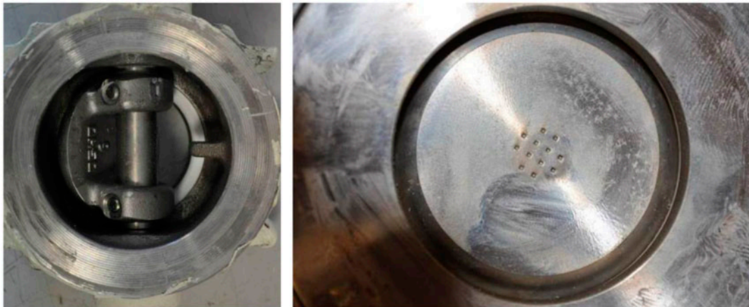
Fig. 11. Photographs of butterfly valve after one month at impressed potential of -600 mV/SCE.
