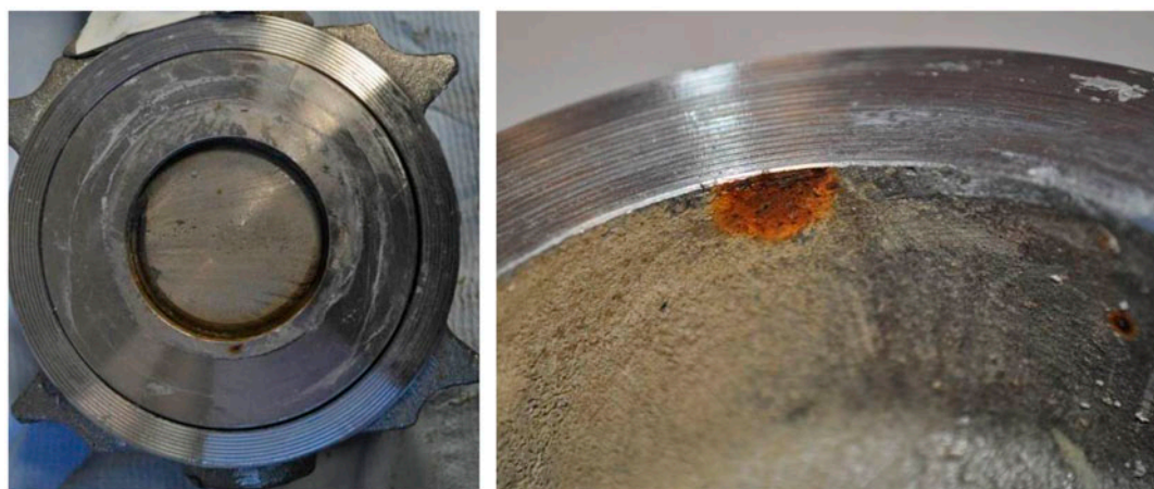
Fig. 10. Photographs of butterfly valve after one month at impressed potential of -400 mV/SCE.
