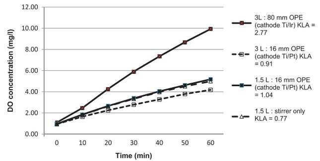
Fig. 5. DO concentration and  $K_{La}$  produced by OPEs of different size (16 mm and 80 mm) with different volumes (1.5 and 3 L) of MilliQ water.
