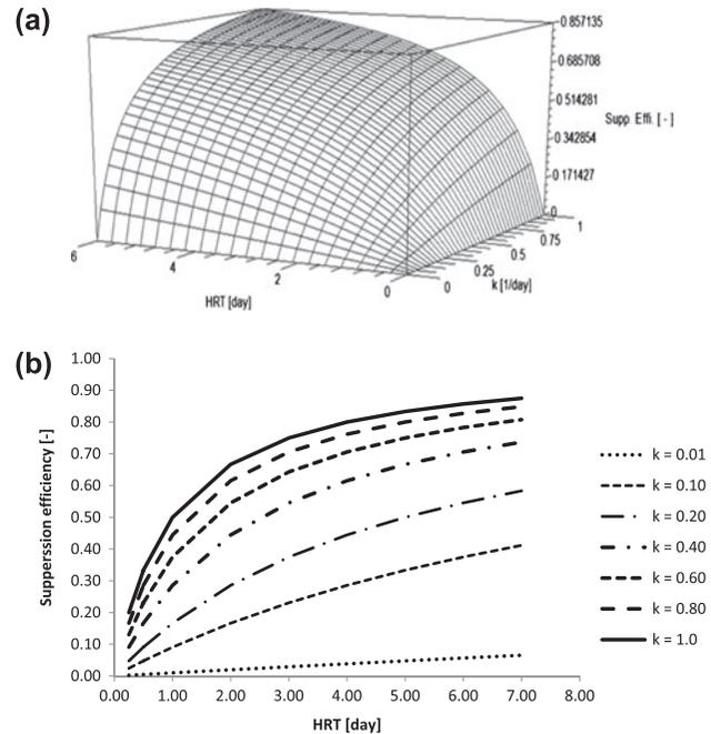
Fig. 2. Suppression efficiencies of single OPE (a) in 3-D graphical form in combination with various  $k$  values and HRTs (b) vs. HRTs with various  $k$  values.
