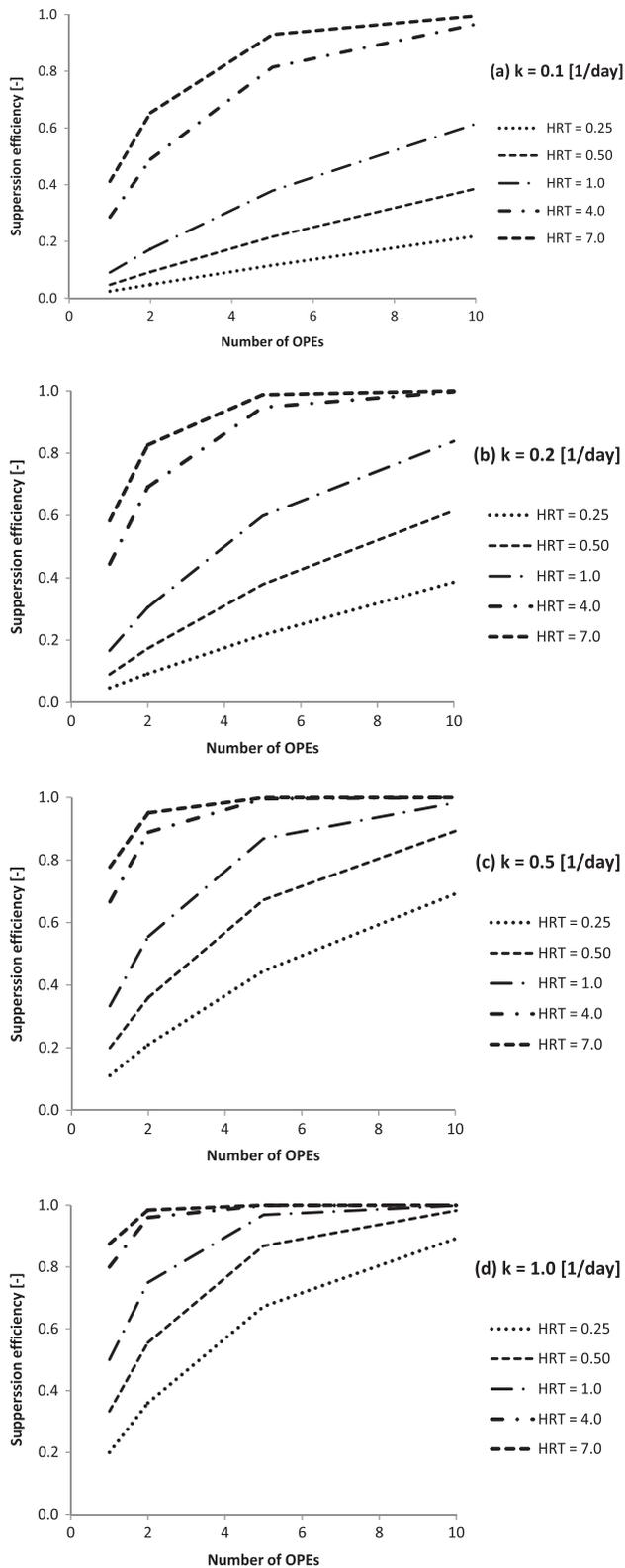
Fig. 3. Suppression ratio with number of OPEs and various HRT at (a)  $k = 0.1$  [1/d] (b)  $k = 0.2$  [1/d] (c)  $k = 0.5$  [1/d] (d)  $k = 1.0$  [1/d].
