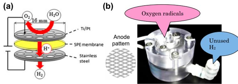
Fig. 1. Pictures of OPE shown A. OPE schematic diagram B. anode pattern (mesh) C. point where radicals are released.
