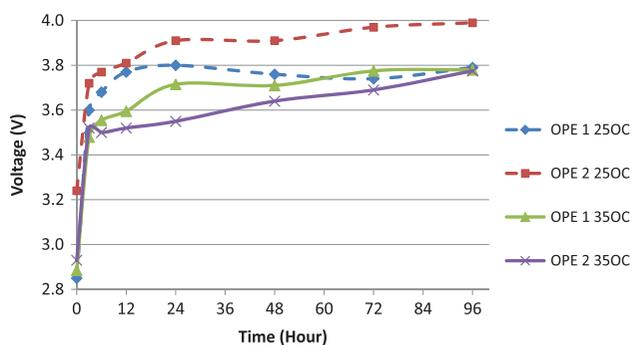
Fig. 6. OPE voltage at 25 and  $35^\circ\text{C}$  for 2 duplicate OPE units, OPE 1 and OPE 2 ( $n = 2$ ).
