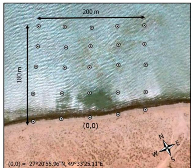
Fig. 2. Sampling points transect for surface bottom sediment analysis.
