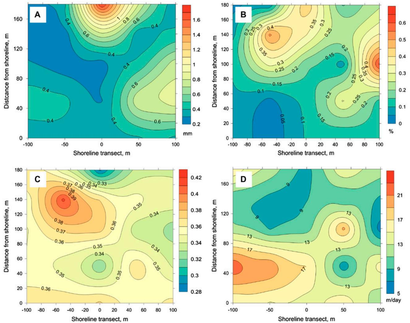
Fig. 4. Unconsolidated bottom surface sediment analyses results mapped in the study area (A) mean grain size, (B) mud percentage, (C) porosity, and (D) hydraulic conductivity.
