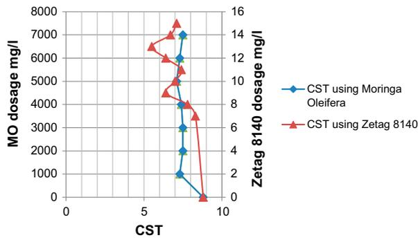
Fig. 1. Capillary suction time (CST) using single polymer.
