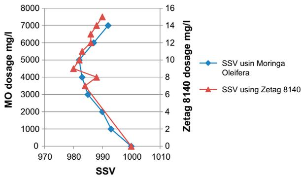
Fig. 7. SSV using single polymer.
