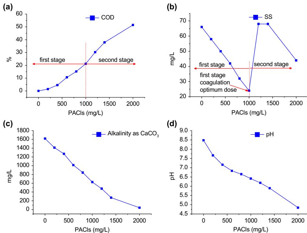
Fig. 2. Water qualities for different PACls dosages in non-adjusting alkalinity jar-test (after biological treatment).
