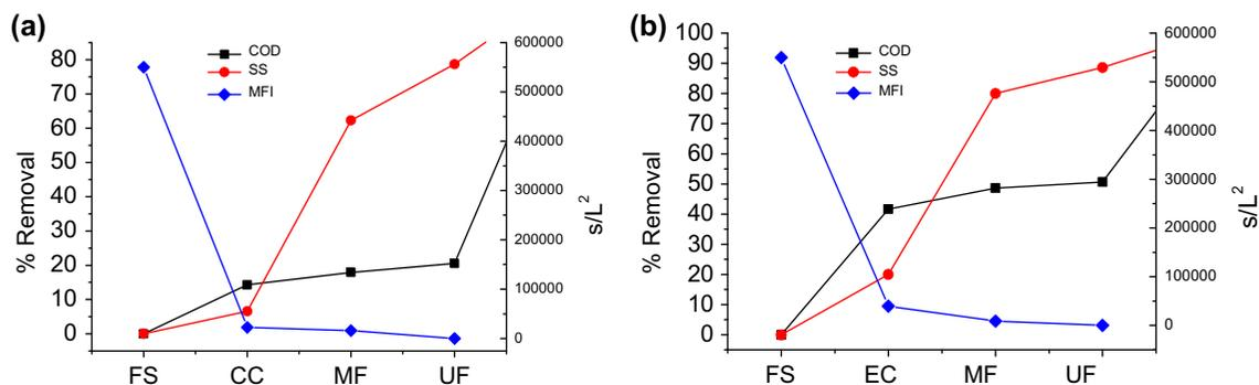
Fig. 4. COD, SS, and MFI for membrane pretreatment processes for (a) CC with MF–UF and (b) enhanced coagulation with MF–UF.
