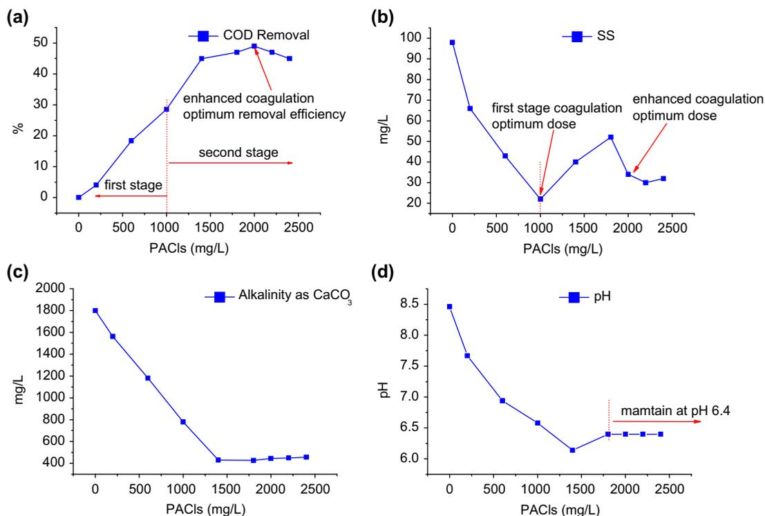
Fig. 3. Water qualities for different PACls dosages in adjusting alkalinity jar-test (after biological treatment).
