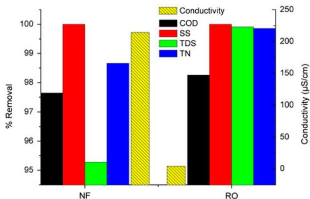
Fig. 6. The variations in electrical conductivity and removal efficiencies of effluent qualities.
