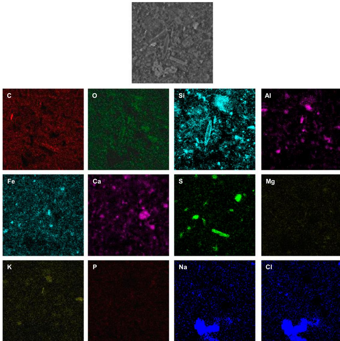
Fig. 5. Elemental mapping for the area of the MFI filter surface without antiscalant treatment shown in Fig. 4(a).
