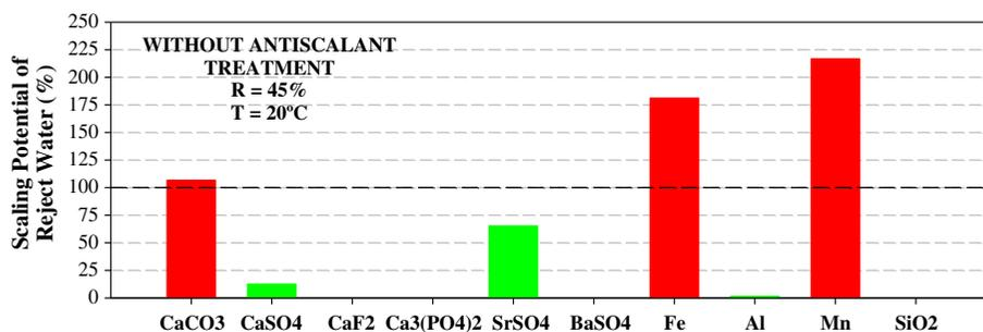
Fig. 7. Scaling potential of rejected water (recovery = 45%) without antiscalant treatment at  $T = 20^{\circ}\text{C}$ .
