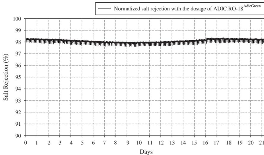
Fig. 9. Normalized salt rejection with the dosage of antiscalant for 21 d of operation.
