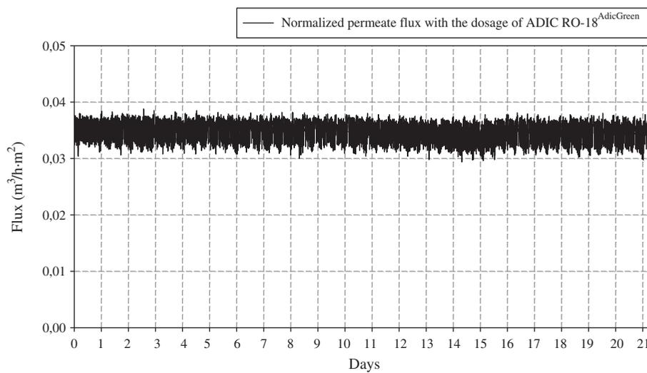
Fig. 8. Normalized permeate flux with the dosage of antiscalant for 21 d of operation.
