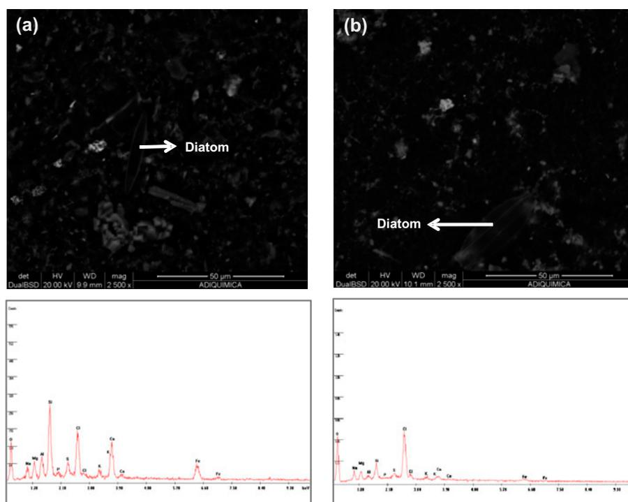
Fig. 4. SEM microphotographs (2500× magnification) and EDX analysis of MFI filter surfaces: (a) without antiscalant treatment and (b) with antiscalant dosage.
