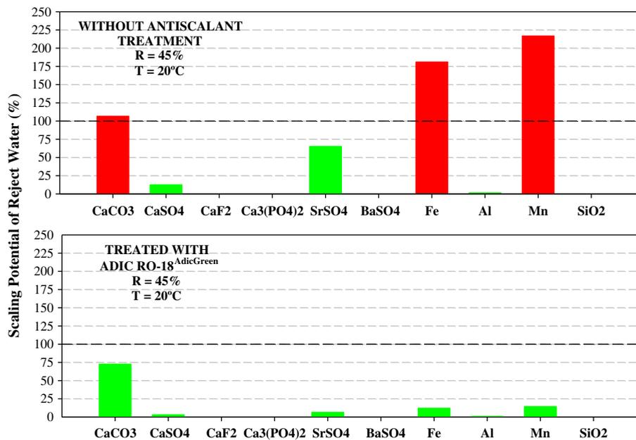
Fig. 12. Scaling potentials of rejected water (recovery = 45%) without and with antiscalant treatment at  $T = 20^{\circ}\text{C}$ .
