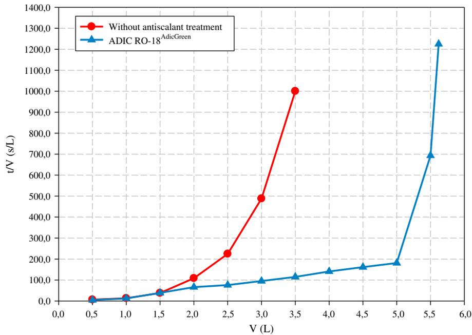
Fig. 1. Filtration curve at constant pressure without and with antiscalant treatment.
