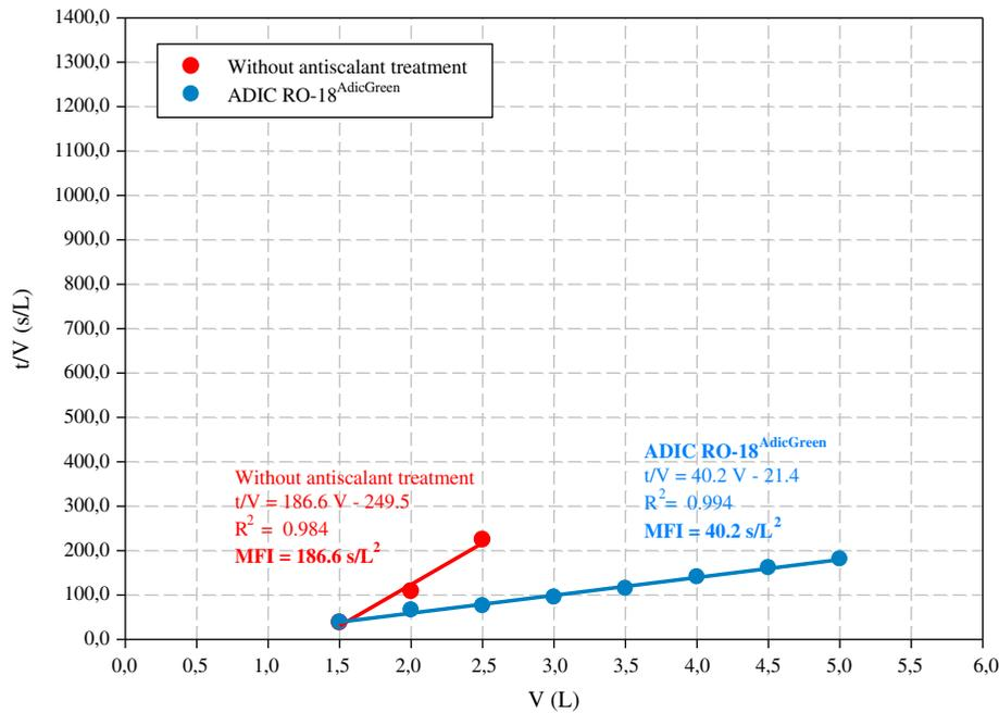
Fig. 2. MFI calculation from filtration curves at constant pressure without and with antiscalant treatment.
