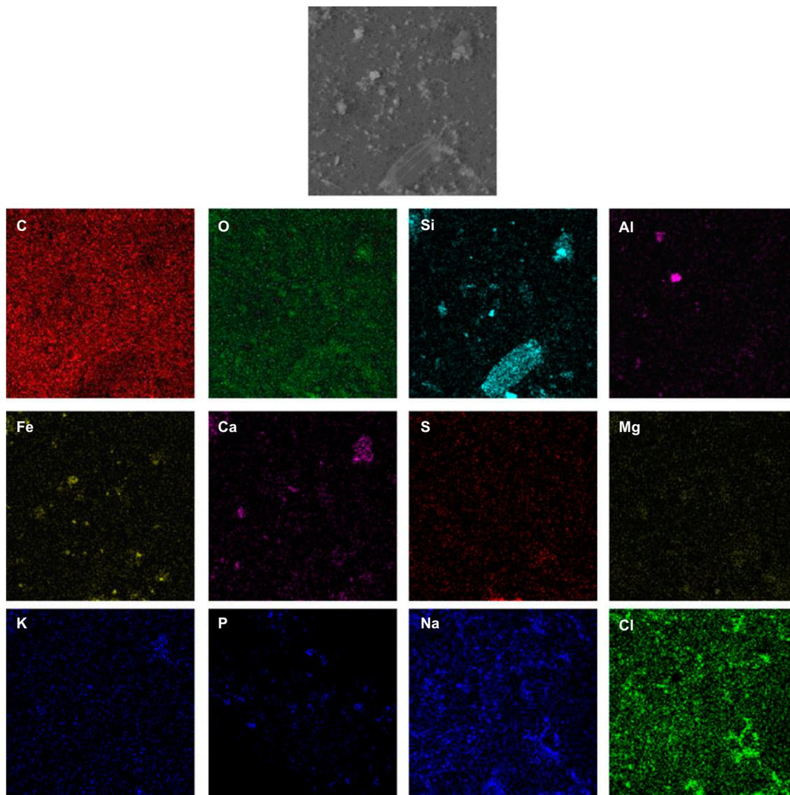
Fig. 6. Elemental mapping for the area of the MFI filter surface with antiscalant dosage shown in Fig. 4(b).
