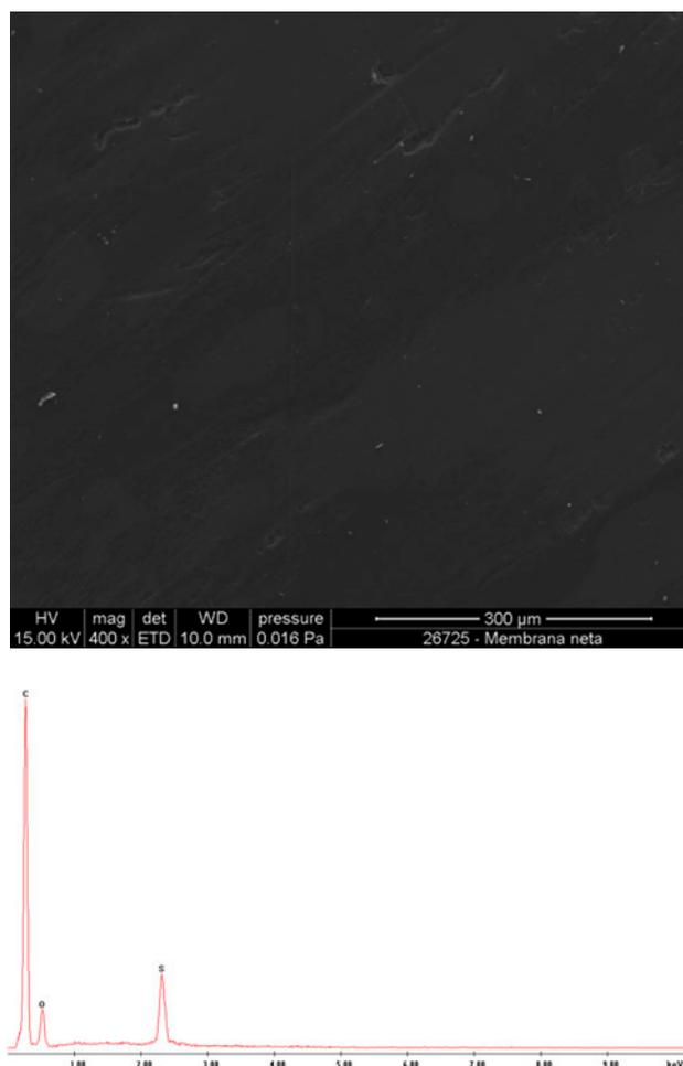
Fig. 11. SEM microphotograph (400× magnification) and EDX analysis of the reverse osmosis membrane surface used during the test with the dosage of antiscalant.
