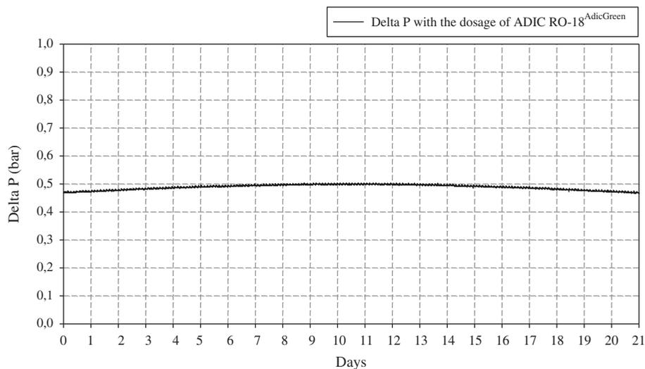
Fig. 10. Delta P with the dosage of antiscalant for 21 d of operation.
