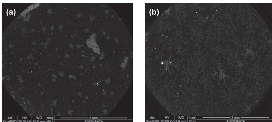
Fig. 3. SEM images of MFI filter surfaces (50× magnification): (a) without antiscalant treatment and (b) with antiscalant dosage.
