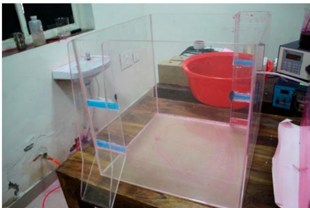
Fig. 1. An acrylic wetland model with dimension of 50 cm × 50 cm × 50 cm.
