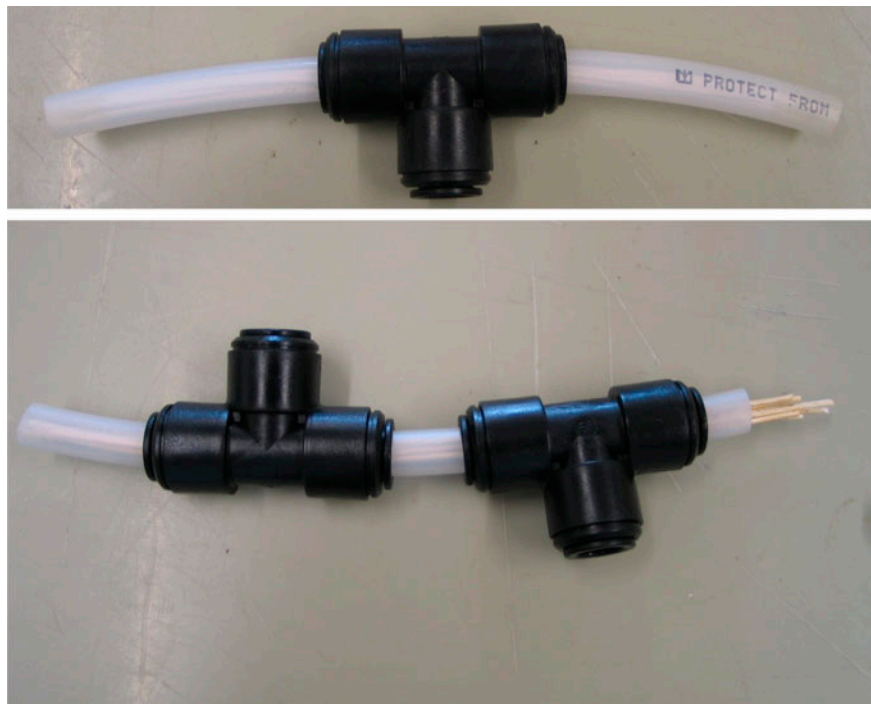
Micromodules for UF fibre testing. Top picture shows an “in to out” module, bottom picture shows an “out to in” module
