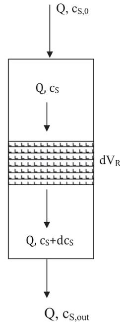
Fig. 5. Scheme of a tubular bioreactor with packed bed.
