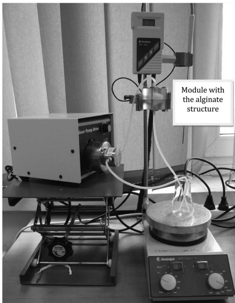
Fig. 2. Set of apparatus for determining kinetics of an encapsulated enzyme.
