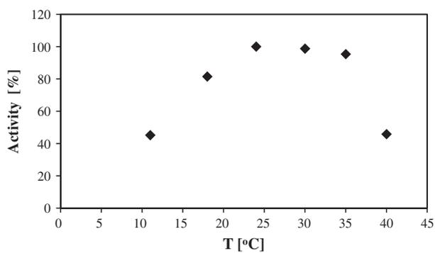
Fig. 3. The temperature profile of catalase immobilized in alginate capsules (pH 6.4). 100% activity corresponds to the activity at 24°C.
