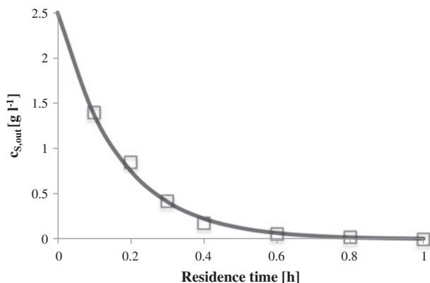
Fig. 6. The outlet concentration of substrate vs. residence time (experimental—points, model-line).
