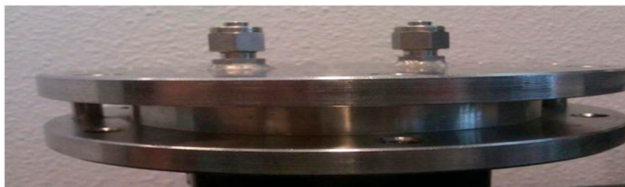
Fig. 4. Side view of Setup 1 (upper: feed chamber, lower: distillate chamber).
