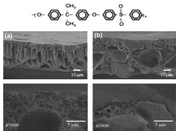
Fig. 1. SEM pictures of cross-section of (a) PSf and (b) HMIP membrane embedded for BPA-imprinted polymer powders.
