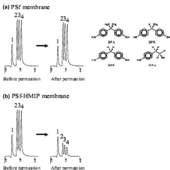
Fig. 2. HPLC charts of aqueous solution containing HPA (1), BPF (2), BPE (3), and BPA (4) before and after permeation by the PSf and PSf-HMIP membrane.
