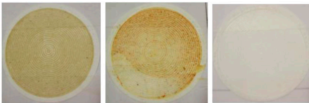
Fig. 1. SDI 15 filter for raw water, conventional treatment outlet, and UF unit filtrate.
