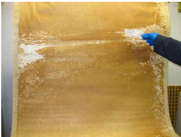
Fig. 7. Foulant on membrane sheet.
