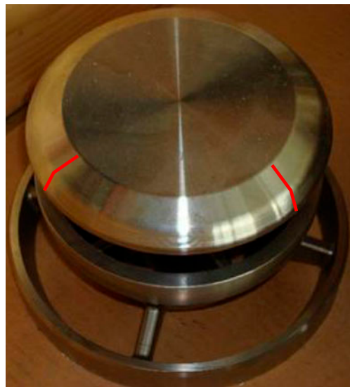
Fig. 8. Check valve disc with updated profile.
