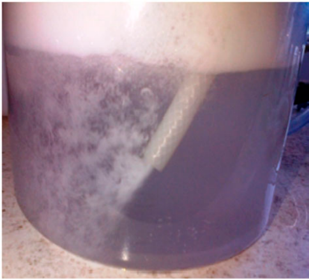
Fig. 2. Small refined bubbles with Cleaner A + air.
