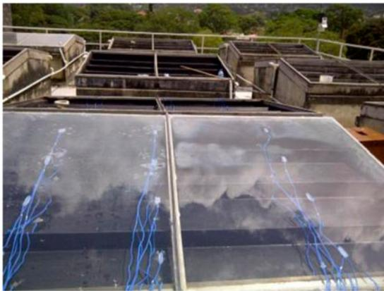
Fig. 2. Picture depicting the thermocouples fixed onto the inner glass surface.
