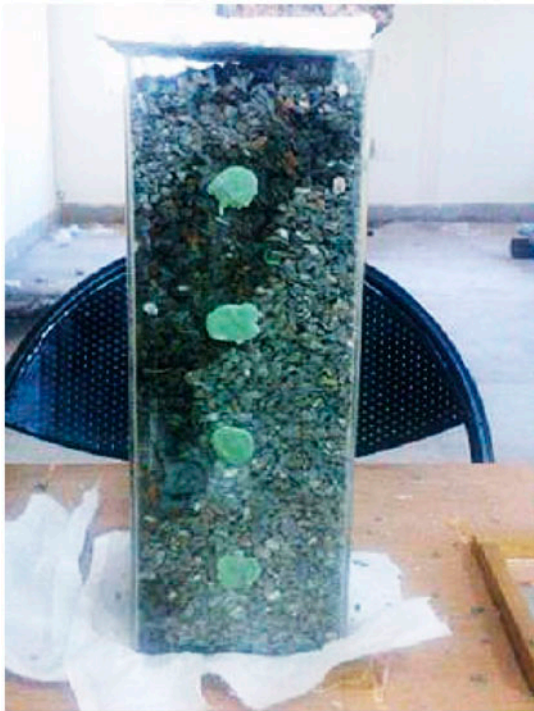
Fig. 1. Thirty centimetre acrylic column filled with gravels of average size 6 mm.
