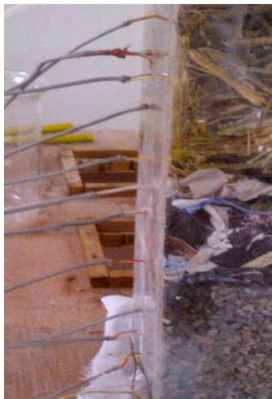
Fig. 8. Thermocouples inserted in the multi-media-layered reactor.
