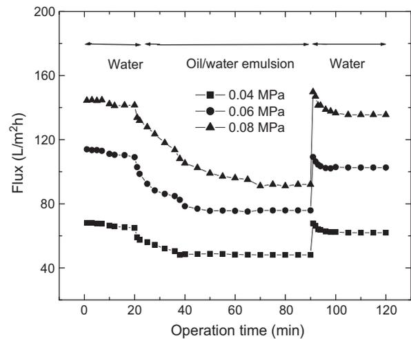
Fig. 9. The influence of operation pressure on water permeate fluxes of the fluorinated membrane as a function of operation time.
