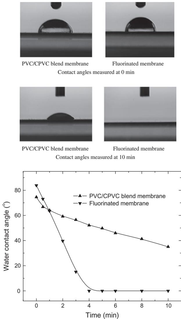
Fig. 5. (Top) Photographs of water contact angles measured at 0 and 10 min. (Bottom) The relationship between water contact angles of PVC/CPVC blend membrane and the fluorinated membrane as a function of measurement time.
