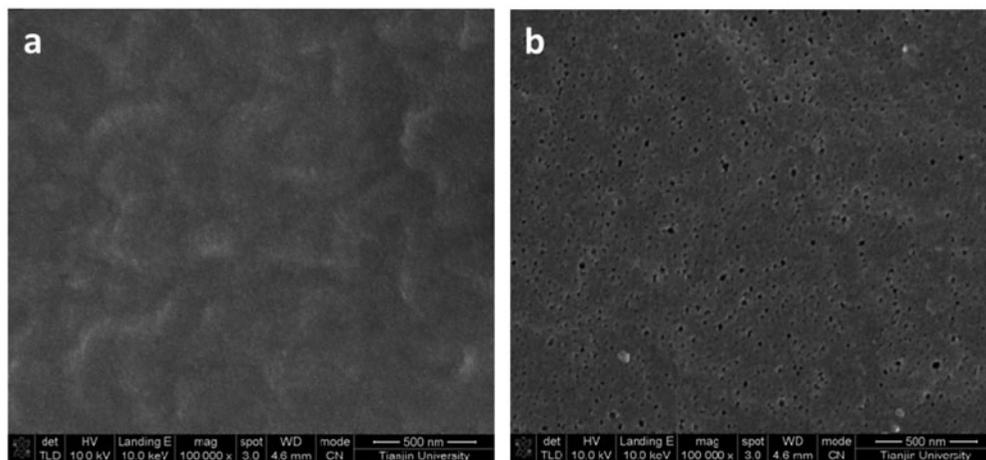
Fig. 10. Morphology of membrane surface after fouling experiment: (a) PVC/CPVC blend membrane; (b) the fluorinated membrane.
