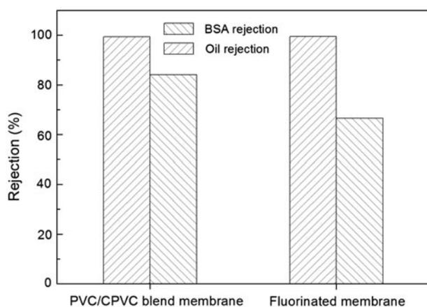
Fig. 7. The BSA and emulsified oil droplets rejection ratios of PVC/CPVC blend membrane and the fluorinated membrane.
