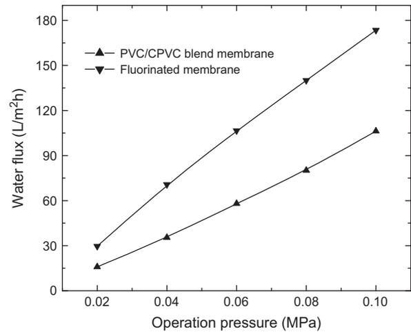
Fig. 6. Pure water fluxes of PVC/CPVC blend membrane and the fluorinated membrane as a function of operation pressure.
