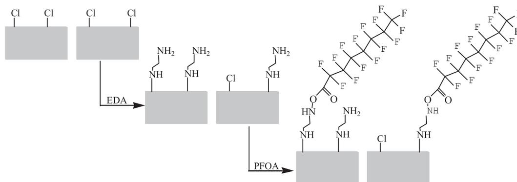
Fig. 1. Schematic illustration of grafting perfluoroalkyl groups onto PVC/CPVC blend membrane surface for preparing the fluorinated membrane.
