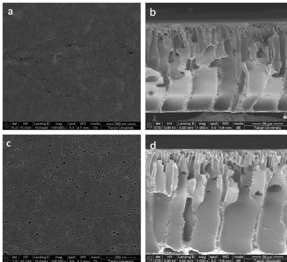
Fig. 2. The surface and cross-section SEM morphologies of (a, b) PVC/CPVC blend membrane and (c, d) the fluorinated membrane.
