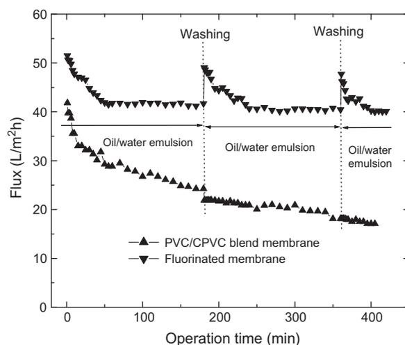
Fig. 8. Water permeate fluxes of PVC/CPVC blend membrane and the fluorinated membrane as a function of operation time in oil/water emulsion separation at pressure of 0.04 MPa. The membranes were cleaned by water at time of 180 and 360 min, and reused in the oil/water emulsion separation.
