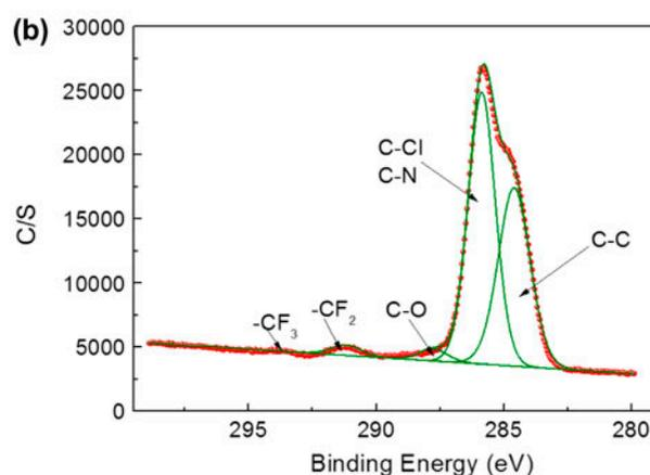
Fig. 4. (a) XPS spectra of the fluorinated membrane; (b) C1s core level spectra resolving results of the fluorinated membrane.
