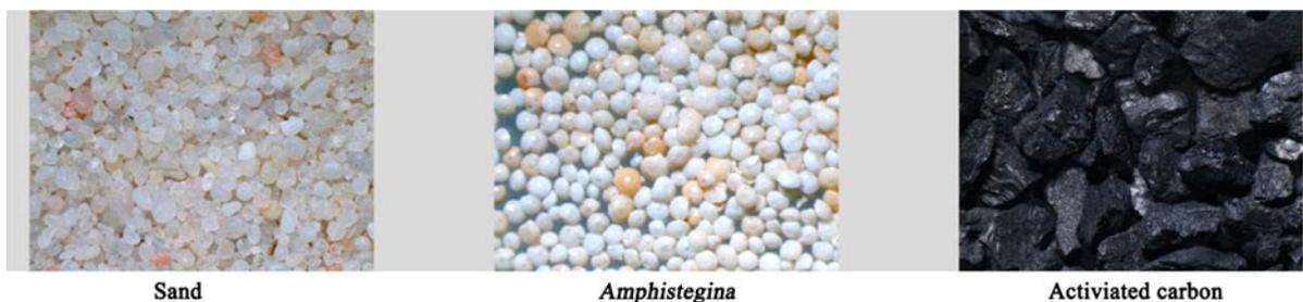
Fig. 1. Photomicrographs of filter media used in the vessels.
